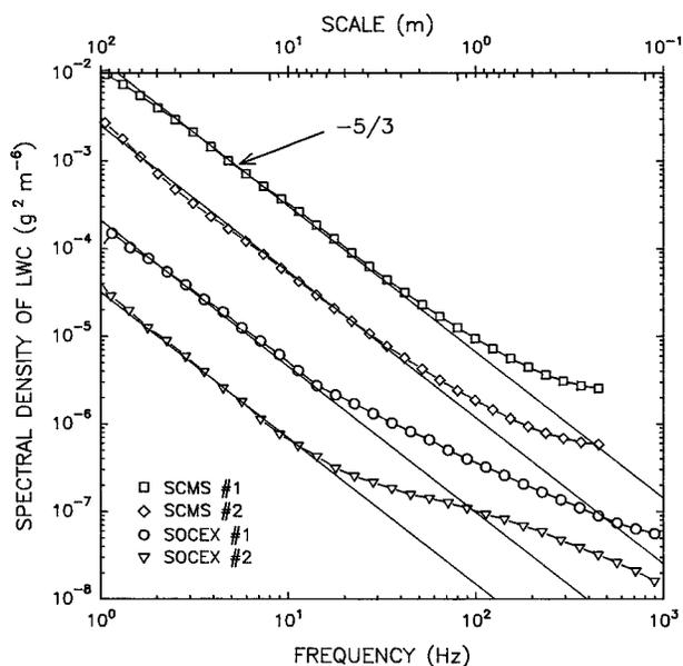
FIG. 3. Relative values of the spectral density of LWC measured during horizontal passes through two clouds in the SOCEX and in the SCMS experiments are compared to the  $-5/3$  scaling law. Shifted scales shown on the SCALE axis apply to the SCMS aircraft speed of  $100 \text{ m s}^{-1}$  (upper scale) and to the SOCEX aircraft speed of  $80 \text{ m s}^{-1}$  (lower scale).
