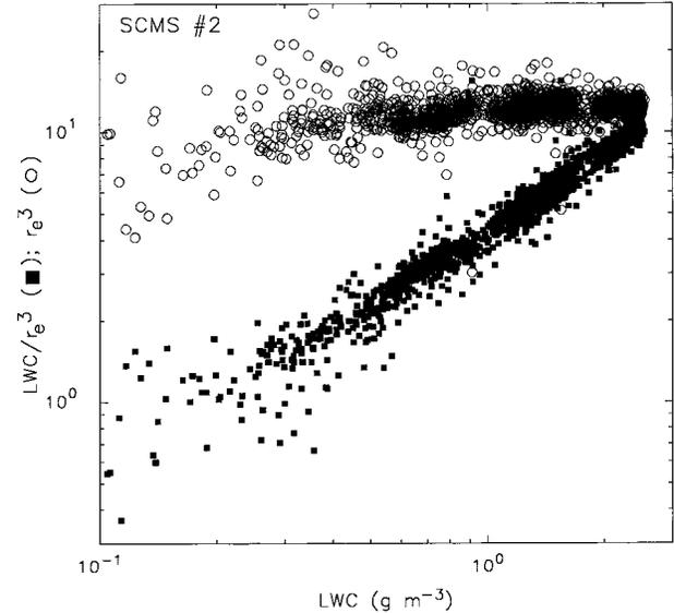
FIG. 2. The relative concentrations of cloud droplets estimated by  $LWC/r_e^3$ , and relative values of  $r_e^3$  as a function of LWC measured simultaneously at 250 Hz (40-cm resolution) by the PVM in Cu cloud-pass SCMS #2 on 22 Jul 1995. No attempt has been made to identify and exclude 250-Hz samples that are part cloudy, part clear air.
