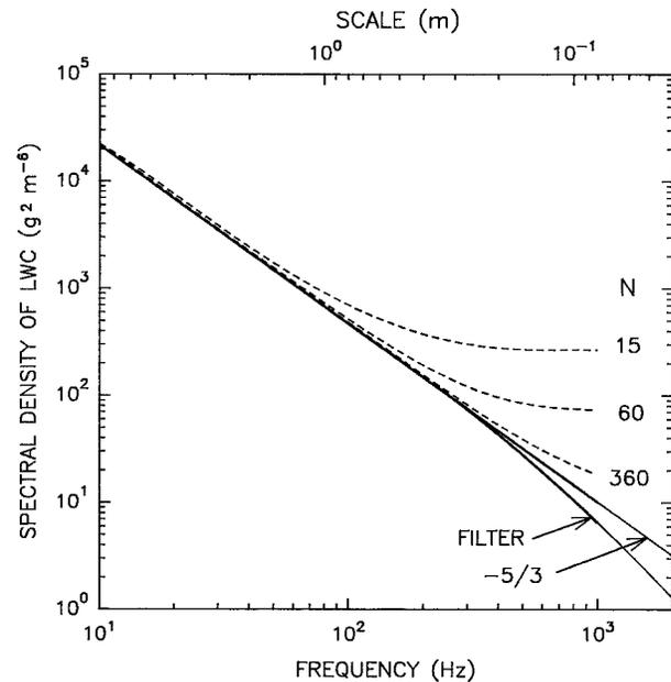
FIG. 1. Predicted statistical sampling noise (dashed curves) in the spectral density of LWC for  $N$  number of monodisperse droplets in the sampling volume of the PVM. The variability of LWC follows the  $-5/3$  scaling law (straight solid line), and the droplets are spatially distributed according to the Poisson law. The effect of the low-pass filter in the PVM is also shown (see text).
