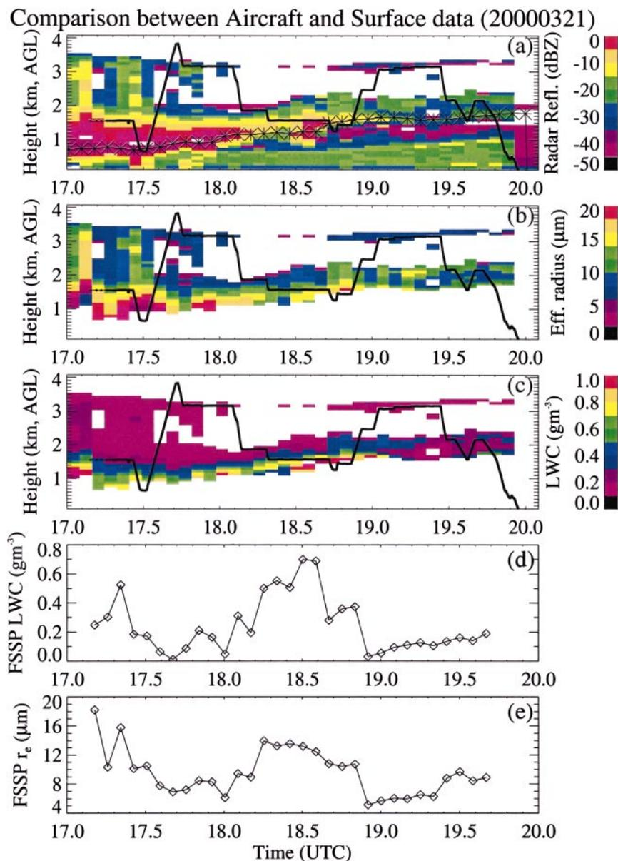
FIG. 9. (a) Radar reflectivity with ceilometer-measured cloud-base height (asterisks), (b) cloud  $r_e$ , and (c) LWC profiles (5 min). Aircraft altitude (solid line) in (a), (b), and (c). (d) The 5-min averages of cloud LWC and (e)  $r_e$  from the aircraft FSSP data.
