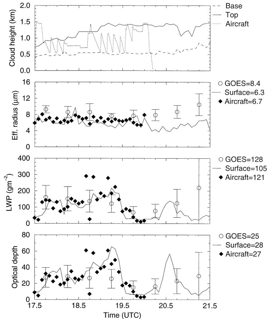
FIG. 4. The ceilometer-measured cloud-base height (dash) and radar-derived cloud-top height (solid),  $r_e$ , LWP, and  $\tau$  vs time for 3 Mar 2000. The means given on the right of the panels represent the averaged values when all three datasets are available, such as from 17.5 to 20.0 UTC.
