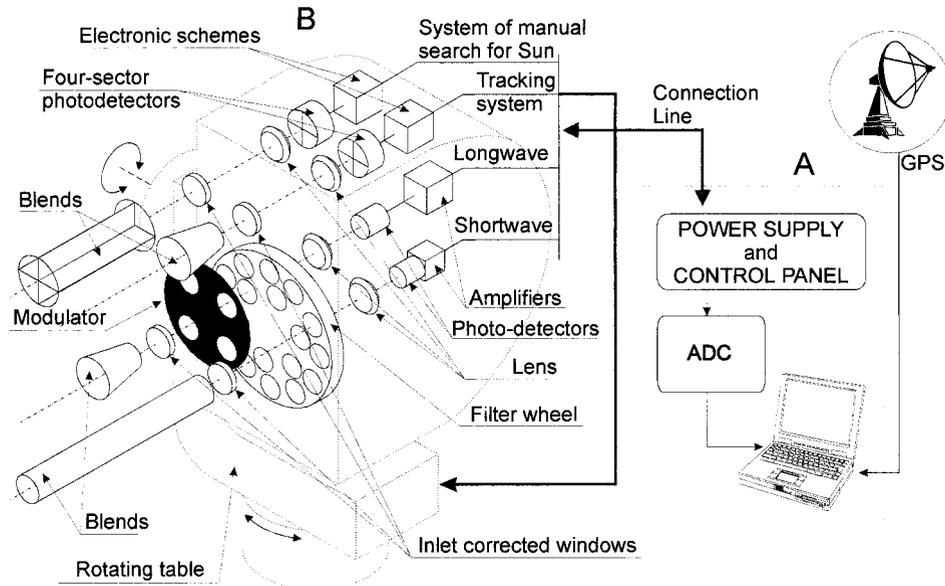
FIG. 2. Scheme of sun photometer SP-3.
