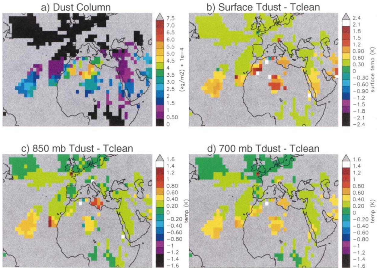
FIG. 11. Differences in temperatures from two types of retrievals on 15 Aug 1988. One retrieval,  $T_{\text{dust}}$ , assumes dust concentrations simulated from the GOCART model. (a) The GOCART simulated aerosol column loading. The second retrieval,  $T_{\text{clean}}$  assumes no dust. Retrievals are from simulated TOVS radiances that assume the GOCART dust concentrations. (b)  $T_{\text{dust}} - T_{\text{clean}}$  at earth's surface, (c) at 850 mb and (d) at 700 mb.
