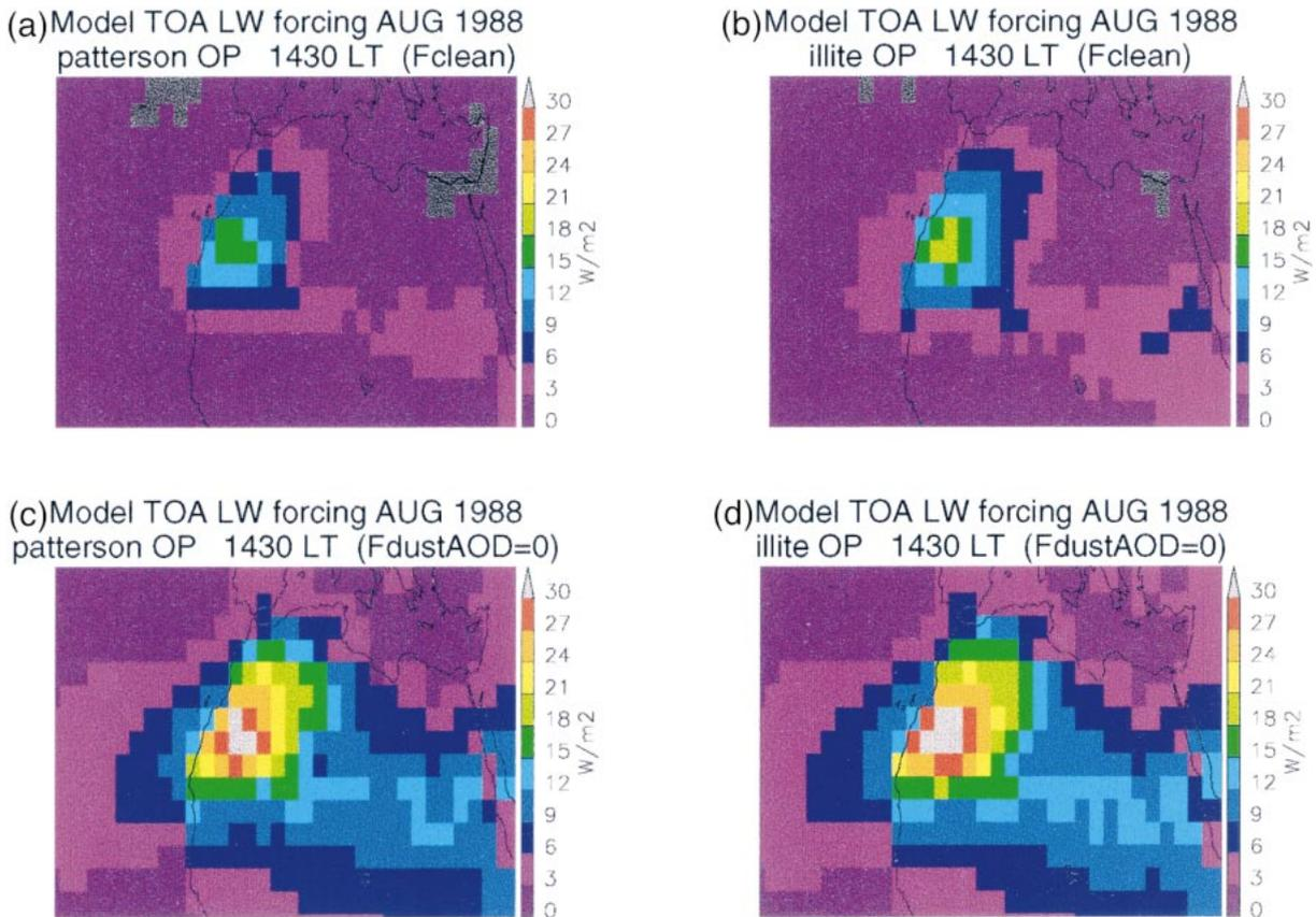
FIG. 6. Monthly mean TOA longwave  $\Delta F_{\downarrow} = F_{\text{dust}\downarrow} - F_{\text{clean}\downarrow}$  for Aug 1988 using optical parameters from (a) Patterson et al. (1977) and (b) illite. Monthly mean TOA longwave  $\Delta F_{\downarrow} = F_{\text{dust}\downarrow} - F_{\text{dust}\downarrow}$  (AOD = 0) for Aug 1988 using optical parameters from (c) Patterson et al. (1977) and (d) illite. All values are at 1430 LT.
