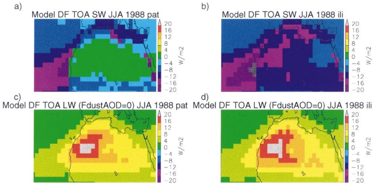
FIG. 7. Average Jun, Jul, and Aug 1988 daily TOA shortwave forcing using (a) Patterson and (b) illite optical parameters. Longwave forcing  $\Delta F_{\downarrow} = F_{\text{dust}\downarrow} - F_{\text{dust}\downarrow}(\text{AOD} = 0)$  using (c) Patterson and (d) illite optical parameters. Positive  $\Delta F_{\downarrow}$  values describe increased incoming or decreased outgoing radiation.
