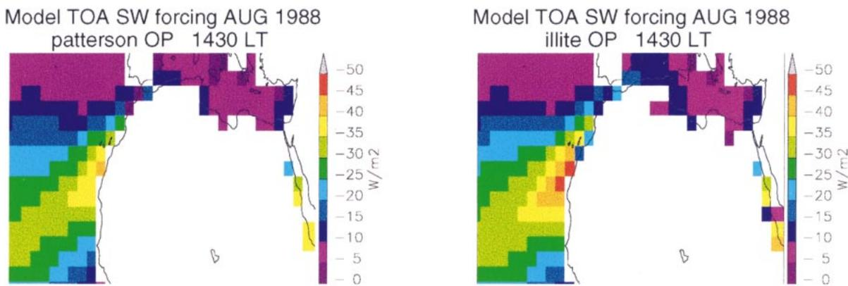
FIG. 4. Monthly mean TOA shortwave  $\Delta F_{\text{dust}} = F_{\text{dust}} - F_{\text{clean}}$  for Aug 1988 using OPs from (a) Patterson et al. (1977) and (b) illite. All values are at 1430 LT.
