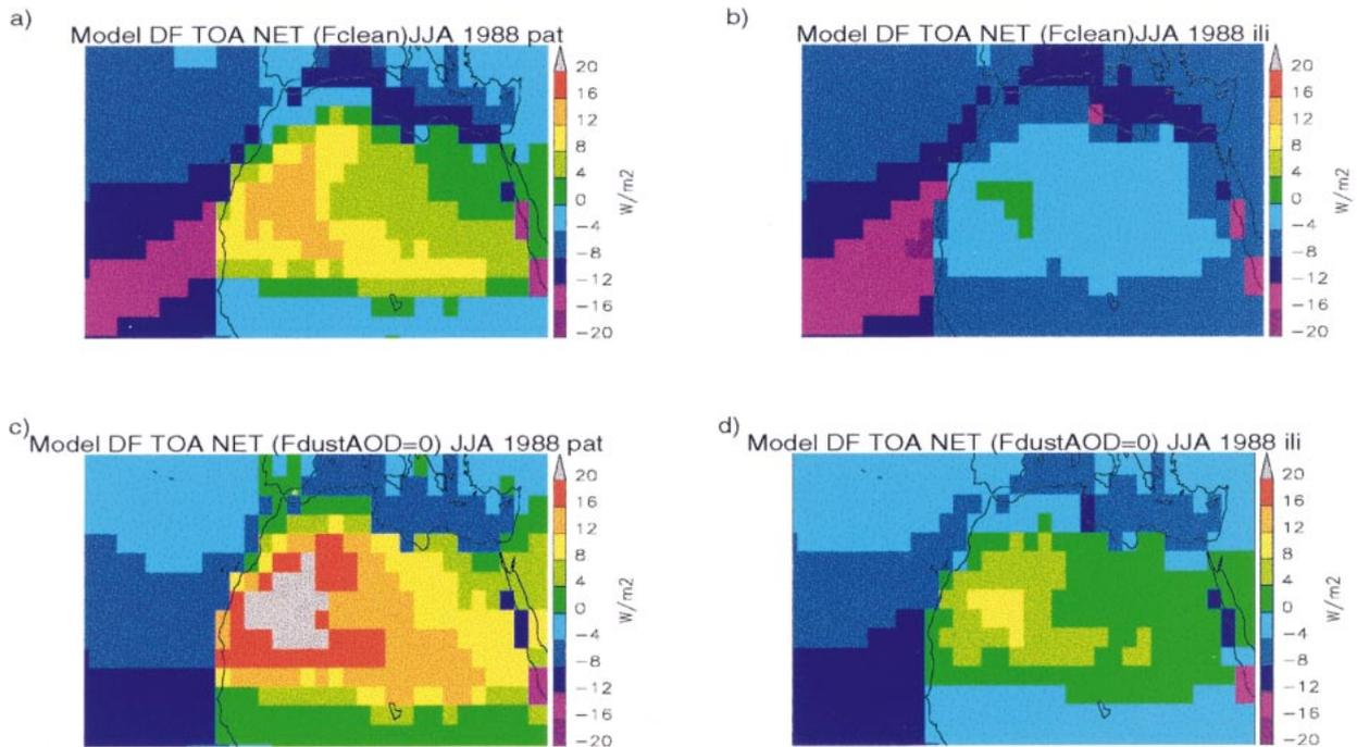
FIG. 8. Average Jun, Jul, and Aug 1988 net TOA forcing. Calculation where LW uses  $\Delta F_{\downarrow} = F_{\text{dust}\downarrow} - F_{\text{clean}\downarrow}$  using (a) Patterson and (b) illite optical parameters. Calculation where LW uses  $\Delta F_{\downarrow} = F_{\text{dust}\downarrow} - F_{\text{dust}\downarrow}$  (AOD = 0) using (c) Patterson and (d) illite optical parameters. Positive  $\Delta F_{\downarrow}$  values describe increased incoming or decreased outgoing radiation.
