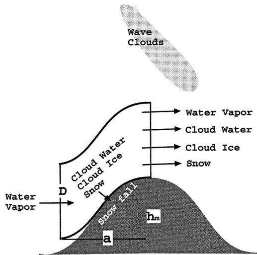
FIG. 3. Sketch of the box model. The box is three-dimensional and includes cloud water, cloud ice, and snow directly produced by mountain upslope lifting.
