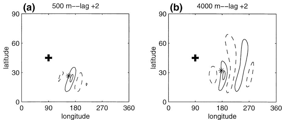
FIG. 6. Eddy meridional wind lag correlations (+2 days) for the (a) 500-m case and (b) 4000-m case. The \* indicates the basis point. Contour interval is 0.2 (zero contour omitted). Dashed contours are negative.
