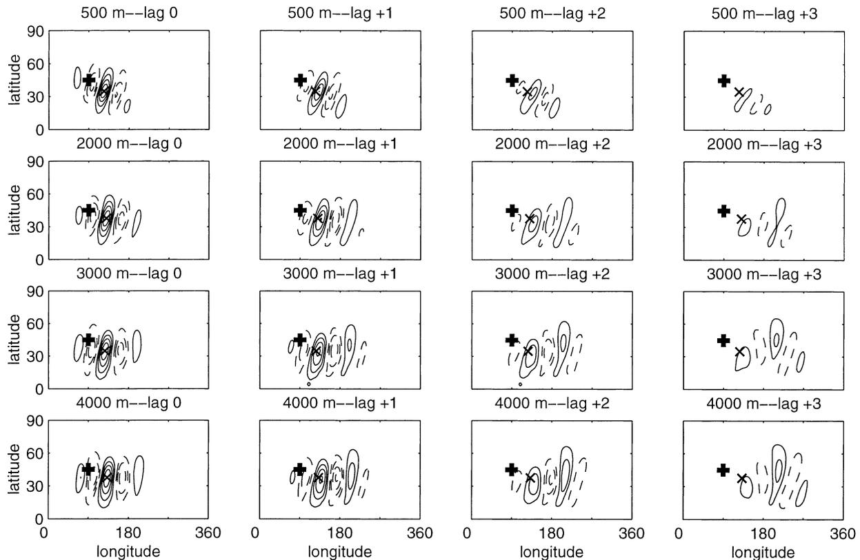
FIG. 5. Eddy meridional wind lag correlations for the (top row) 500-m case, (second row) 2000-m case, (third row) 3000-m case, and (bottom row) 4000-m case. Lags considered are (left-most column) 0 days, (second column) +1 day, (third column) +2 days, and (right-most column) +3 days. The  $\times$  indicates the basis point. Contour interval is 0.2 (zero contour omitted). Dashed contours are negative.
