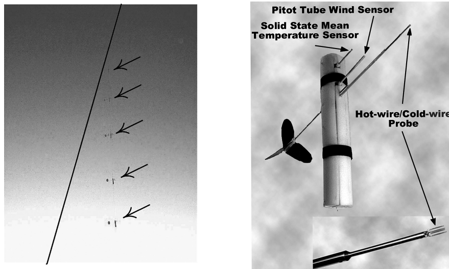
FIG. 1. (left) Photograph of five turbulence probe packages suspended at 6-m intervals below the CIRES TLS during CASES-99. The kite is flying well above the top of the photograph, and the tether is visible as a computer-enhanced straight line to the left of the probes, which are indicated by arrows. (right) Details of a single turbulence sensor package shown in the left.
