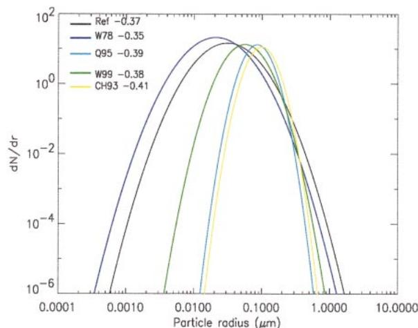
FIG. 2. Size distribution used in the reference calculation and some observations of the accumulation mode. W78 refers to Withby (1978), Q95 to Quinn et al. (1995), W99 to Weingartner et al. (1999), CH93 to Covert and Heintzenberg (1993).
