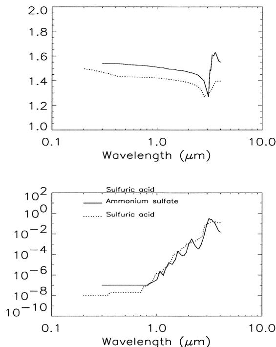
FIG. 3. Refractive index for ammonium sulfate (Toon et al. 1976) and 75% sulfuric acid (Palmer and Williams 1975). (top) Real and (bottom) imaginary refractive index.
