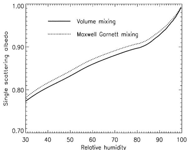
FIG. 7. Single scattering albedo at 550 nm as a function of relative humidity for internal mixing of sulfate and soot with volume mixing and the Maxwell–Garnett mixing.
