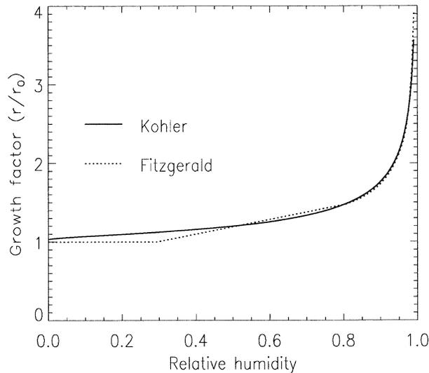
FIG. 4. Growth factor for sulfate aerosols at  $r = 0.05 \mu\text{m}$  based on Fitzgerald (1975) and the Köhler equation.
