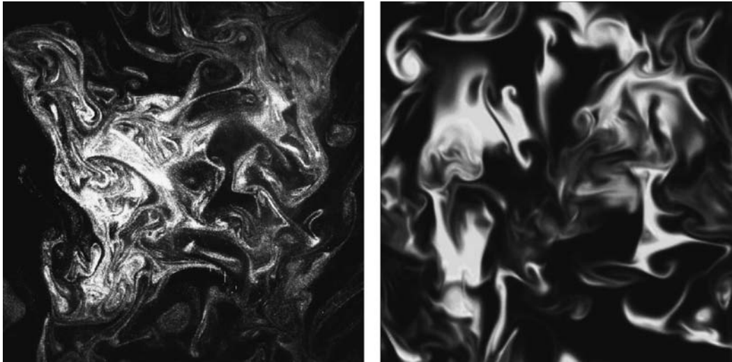
FIG. 4. (right) Vertical cross section from the 256^3 detailed microphysics simulation with low-TKE input at t = 5 s and (left) a laser-sheet photograph of mixing structures observed in the laboratory. Both panels are about 0.6 \text{ m} \times 0.6 \text{ m} . Direction of gravity is from top to bottom.
