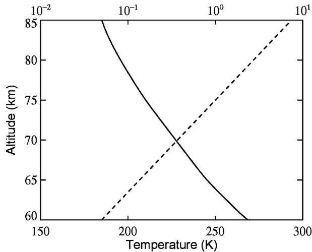
FIG. 3. Profiles of basic temperature (solid) and Newtonian cooling coefficient (dashed) in the Venusian atmosphere adopted in the model.
