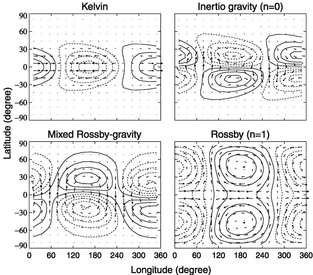
FIG. 6. Same as in Fig. 5, but for test 1. Contour interval is  $40 \text{ m}^2 \text{ s}^{-2}$  for all waves. Arrows are scaled so that the distance occupied by  $10^\circ$  represents 3.9, 8.9, 11.0, and  $5.0 \text{ m s}^{-1}$  for the respective waves.
