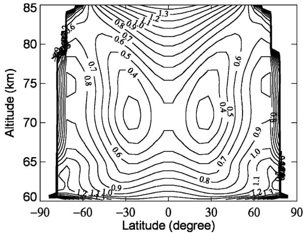
FIG. 8. Meridional distribution of the quasigeostrophic refractive index in the unit of  $\log_{10}(a^2 n_{k,\omega}^2)$  for the Rossby wave in the nominal model. Regions of negative values near the poles are not plotted.
