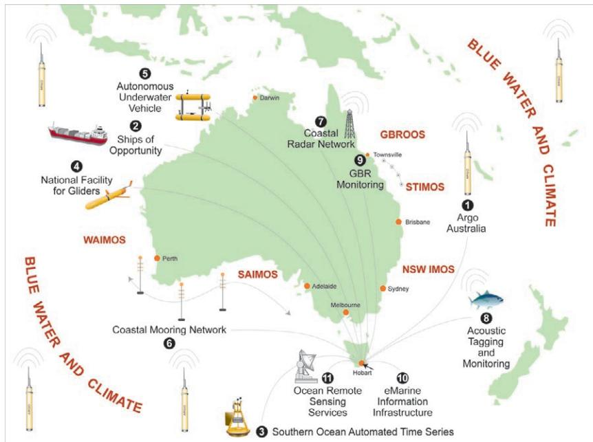
**FIG. 2. Components of the Australian Integrated Marine Observing System (IMOS). Labels with numbers indicate various instrument platforms and infrastructure components. There are five science nodes (in red), one “Blue Water and Climate” node, and four regional nodes. These nodes are responsible for the process of identifying the scientific objectives of various components of IMOS.**
