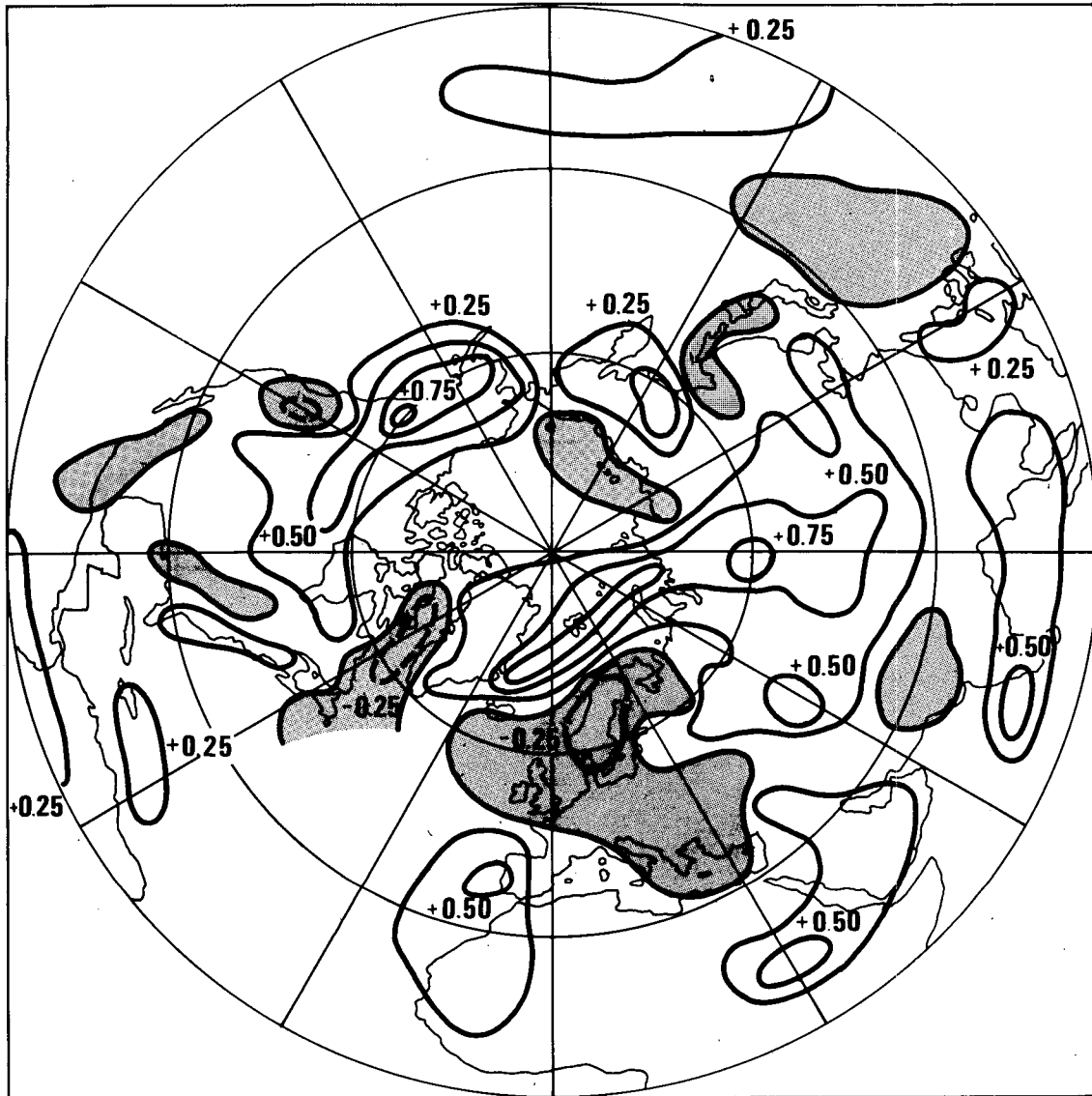
FIG. 2. Linear trend in Northern Hemisphere land-based annual mean surface air temperature over the 1967–86 period. Units ^{\circ}\text{C decade}^{-1} (e.g., +0.25^{\circ}\text{C decade}^{-1} = 0.5^{\circ}\text{C} warming over 1967–86). Shaded areas show cooling. Except where there are suitable islands, most oceanic areas are missing in this analysis.
