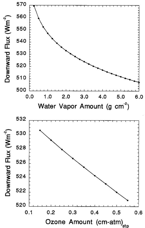
FIG. 1. The downward surface SW flux as a function of the column water vapor amount (upper panel) and ozone amount (lower panel) computed with a solar zenith angle of  $60^\circ$ .
