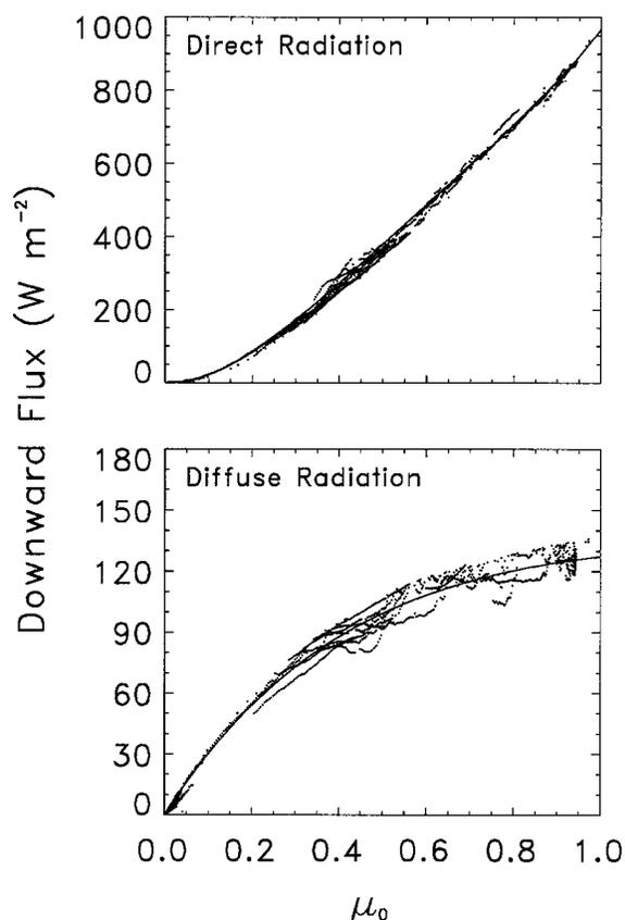
FIG. 6. Estimation of the downward clear-sky SW flux as a function of the cosine of solar zenith angle ( $\mu_0$ ) using method 2 at Kavieng for the four IOP months, November 1992–February 1993. Dots are from surface measurements, and curves are polynomial fits to data points.
