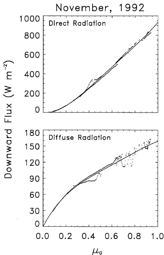
FIG. 2. Estimation of the downward clear-sky SW flux as a function of the cosine of solar zenith angle ( $\mu_0$ ) using method 1 at Kavieng for January 1992. Dots are from surface measurements, and curves are polynomial fits to data points.
