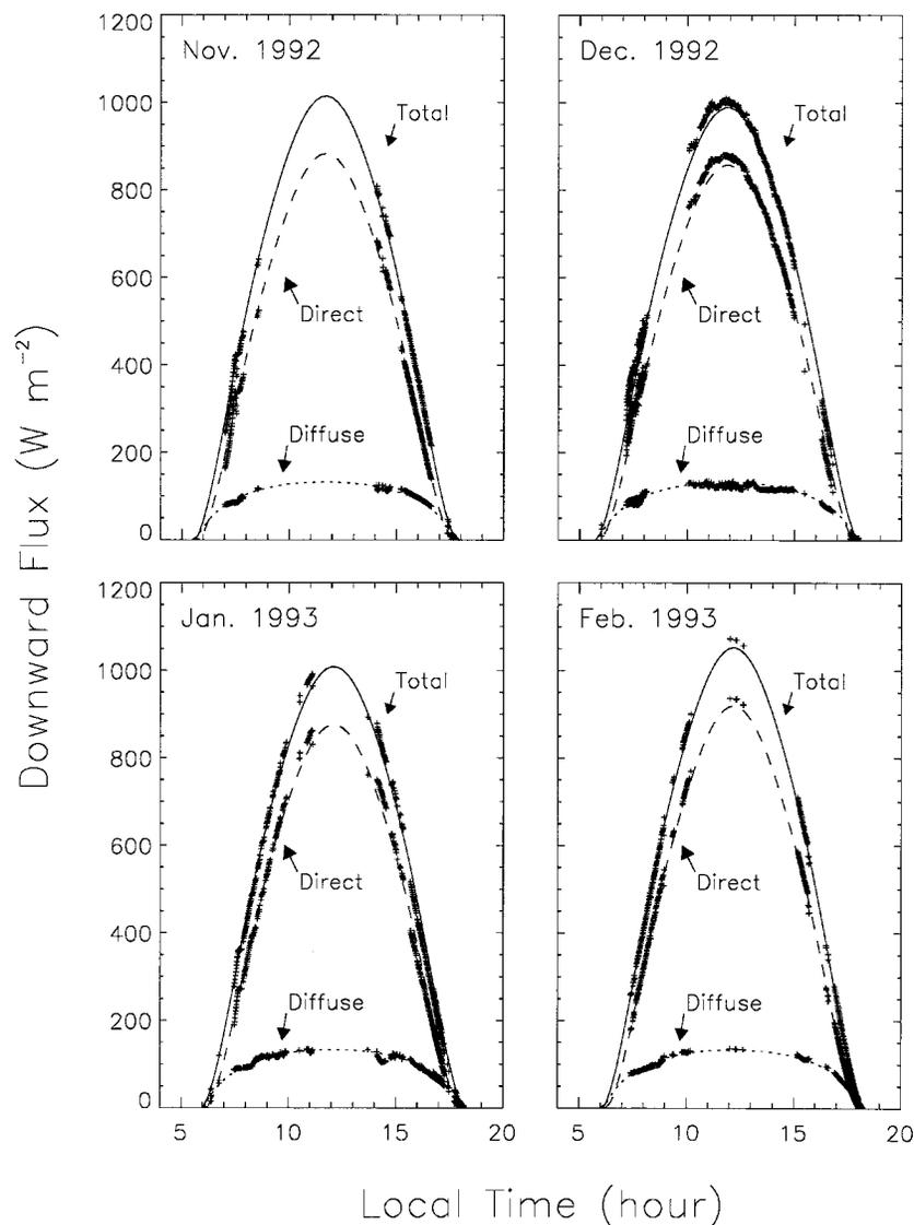
FIG. 9. Monthly mean diurnal variations of the clear-sky downward SW fluxes at Kavieng estimated using method 2. Dots are 1-min clear-sky measurements, and the curves are regressions corresponding to the curves in Fig. 6.
