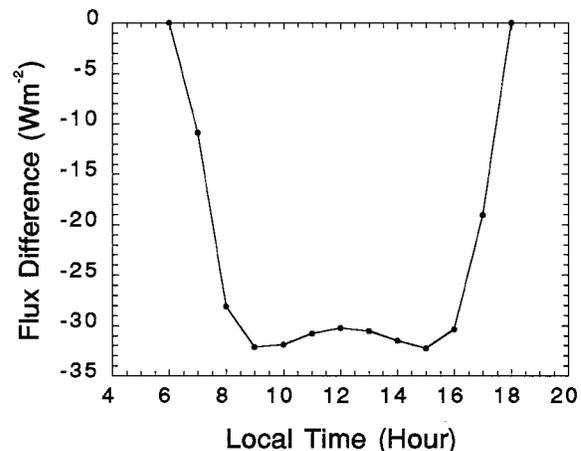
FIG. 11. Diurnal distribution of the aerosol effect on the net downward clear-sky surface SW flux at Kavieng for February 1993. The aerosol optical thickness, single-scattering albedo, and asymmetry factor are set at 0.12, 0.995, and 0.5, respectively.
