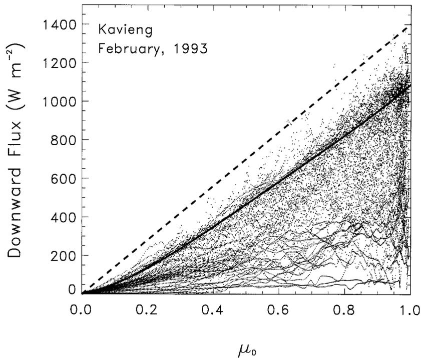
FIG. 8. The total downward SW flux measured at Kavieng for February 1992. Dots are 1-min resolution measurements, the dashed curve is the insolation at the top of the atmosphere, and the solid curve is the estimated clear-sky flux using method 2.
