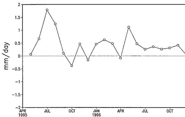
FIG. 10. Differences in  $\langle P - E \rangle$  computed from Eta Model subsampled at the radiosonde temporal and spatial resolution and full Eta Model resolution (in  $\text{mm day}^{-1}$ ).
