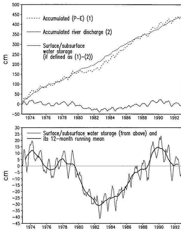
FIG. 7. Time series of accumulated monthly  $\langle P - E \rangle$  and accumulated river discharge for the central United States and their difference (top); the relative storage, thin line, and 12-month running mean of relative storage, heavy line, on an expanded scale (bottom). Units are cm.
