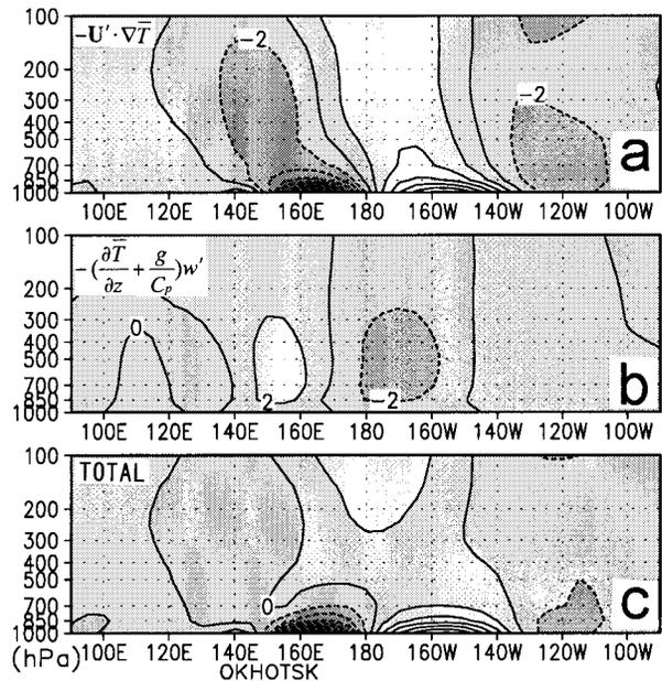
FIG. 8. As in Fig. 6, but for (a) the advection of the basic-state temperature by horizontal wind anomalies, (b) adiabatic heating associated with anomalous vertical motion, and (c) the sum of (a) and (b). Units:  $^\circ\text{C day}^{-1}$ .
