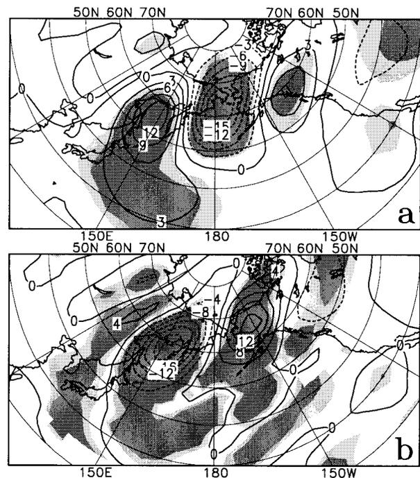
FIG. 4. AGCM response for Jan–Feb mean in (a) sea level pressure (hPa) and (b) surface air temperature ( $^{\circ}\text{C}$ ) to the Okhotsk sea-ice anomalies. Each of the difference maps has been obtained by subtracting the composite response for the five light-case simulations from that for the five heavy-case ones. Areas of light and heavy shading indicate the differences with 95% and 99% confidence levels, respectively, based on the  $t$  statistic (after Honda et al. 1996).
