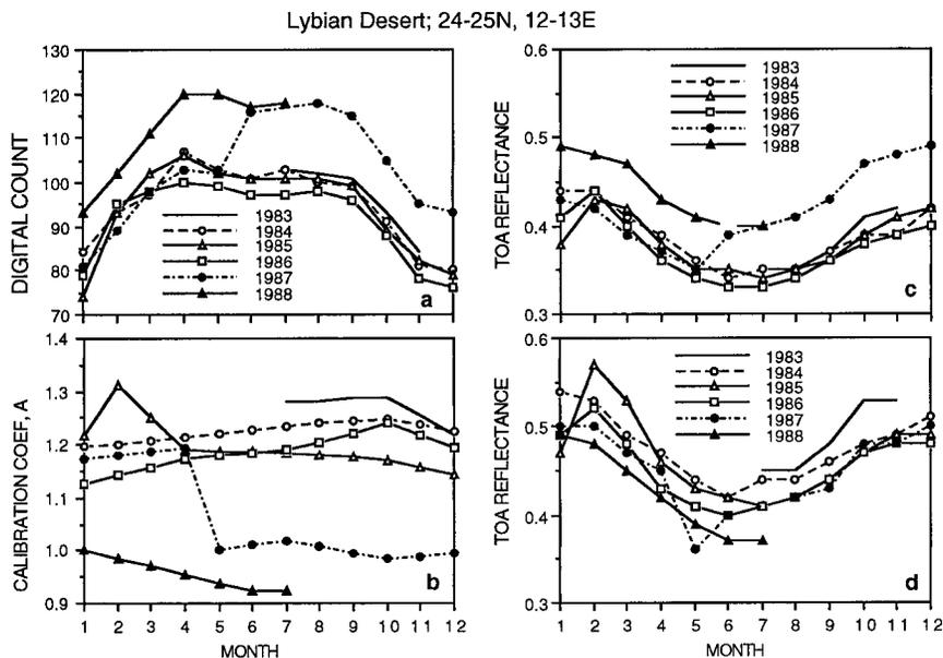
FIG. 1. Monitoring of the Meteosat 2 solar channel over the Libyan desert site. (a) Time series of clear-sky digital count, (b) time series of the ISCCP calibration coefficients  $A$ , (c) time series of TOA reflectance computed with ESOC calibration, and (d) time series of TOA reflectance computed with ISCCP calibration applied.
