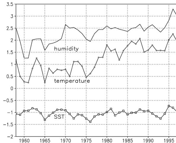
FIG. 5. Anomalies of specific humidity ( $\text{g kg}^{-1}$ ) and temperature (K) at 1000 mb from radiosonde data and SST (K) for the seven best stations. Curves have been shifted vertically to facilitate comparison.
