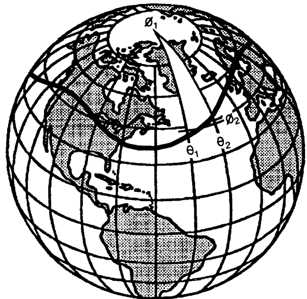
FIG. 1. A simplified representation of the circumpolar vortex area measurement scheme. The vortex (shown here by the heavy black line) is represented by a series of latitude and longitude intersections that are used to define the element bounded north and south by the North Pole ( \phi_1 ) and the average colatitude of the vortex sector ( \phi_2 ), and west and east by the longitude intersections of the sector ( \theta_1 and \theta_2 ).
