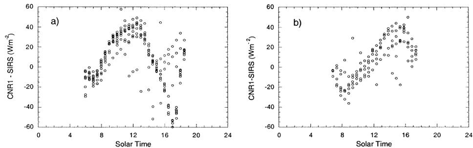
FIG. 13. The diurnal cycle of differences between the K&Z CNR1 and ARM SIRS for incoming shortwave during (a) 11–20 Aug 1999 and (b) 24 Feb–4 Mar 2000.
