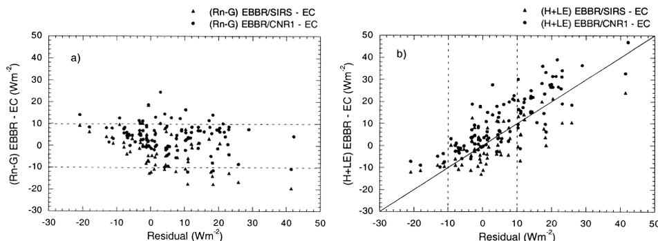
FIG. 4. Daily closure residuals at the EC site as a function of EBBR minus EC measurement differences of (a)  $R_n - G$  and (b)  $H + LE$ . Filled circle data points denote when the BR calculations of  $R_n$  used EC CNR1 measurements (see text).
