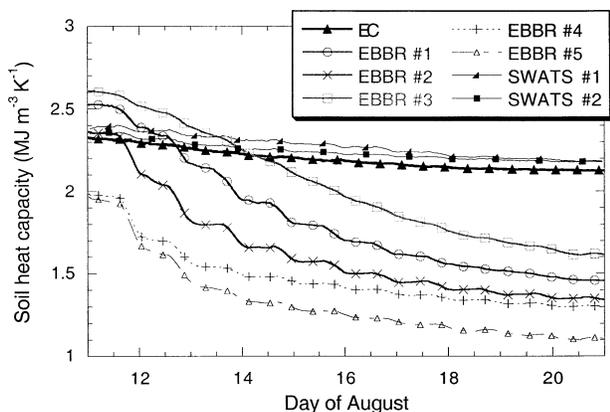
FIG. 15. Daily average values of soil heat capacity estimated as a function of soil moisture data collected from EC, EBBR, and SWATS. Data were collected from 11–20 Aug 1999.
