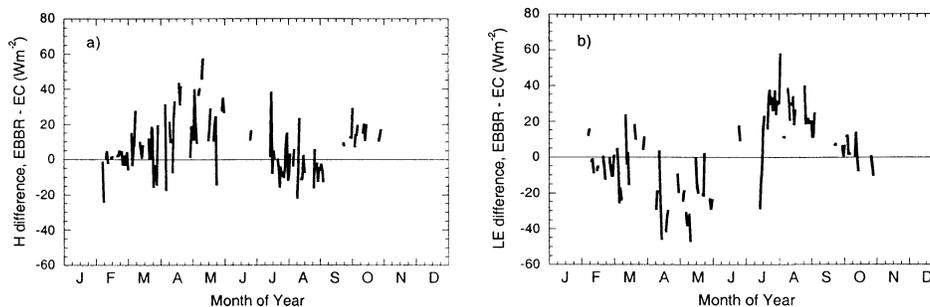
FIG. 7. Differences in daily total (a) sensible heat flux and (b) latent heat flux between the EBBR and EC sites during an annual cycle. Data were collected between 1 Jun 1999 and 31 May 2000.
