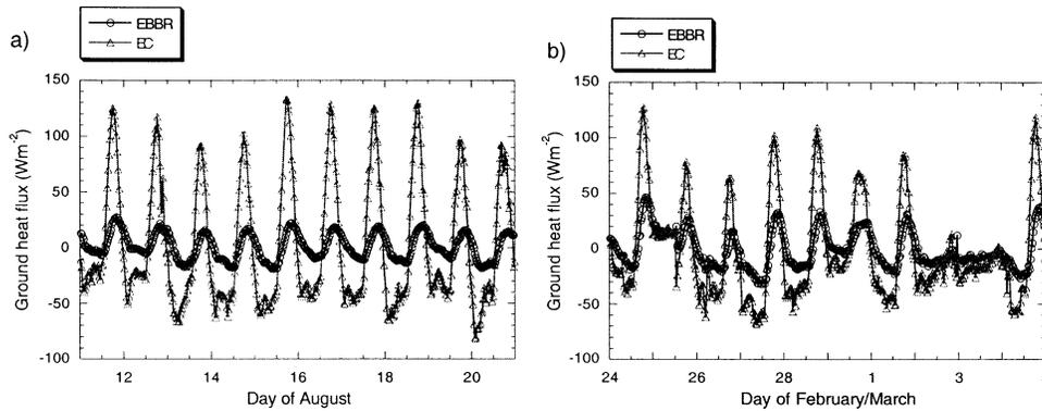
FIG. 19. The time series of the total ground heat flux ( $\text{W m}^{-2}$ ) as measured during (a) 11–20 Aug 1999 and (b) 24 Feb–4 Mar 2000.
