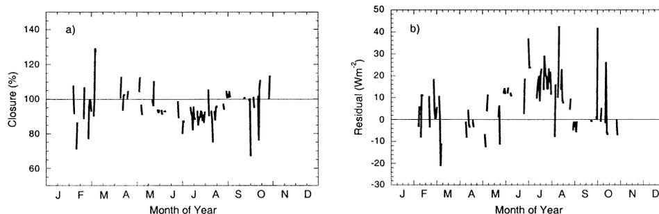
FIG. 2. At the EC site, (a) closure (%) and (b) residual ( $\text{W m}^{-2}$ ) of the energy balance plotted as a function of the day of the year.
