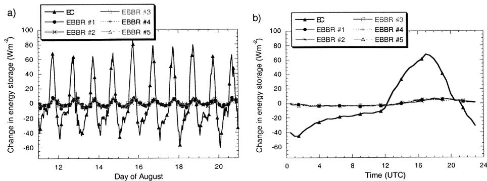
FIG. 18. (a) Time series and (b) 10-day diurnal average of the change in energy storage ( $W m^{-2}$ ) as measured during 11–20 Aug 1999.
