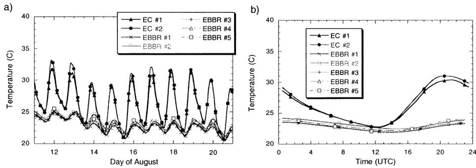
FIG. 17. (a) Time series and (b) 10-day diurnal average of the integrated soil temperature (°C) between 0 and 5 cm as measured by the seven heat flux plates 11–20 Aug 1999.
