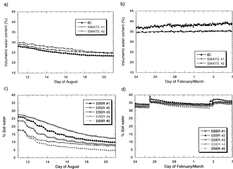
FIG. 14. Volumetric water content (%) as measured during (a) 11–20 Aug 1999 and (b) 24 Feb–4 Mar 2000. Percent soil water as measured during (c) 11–20 Aug 1999 and (d) 24 Feb–4 Mar 2000.
