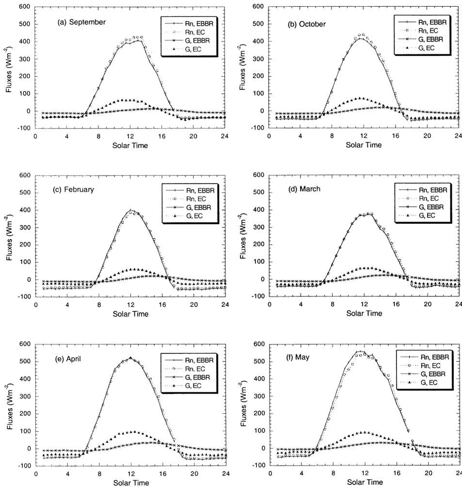
FIG. 9. Monthly mean diurnal cycle of net radiation ( $R_n$ ) and ground heat flux ( $G$ ) as measured at the EBBR and EC sites at Foraker for six different months during 1 Sep 1999–31 May 2000.
