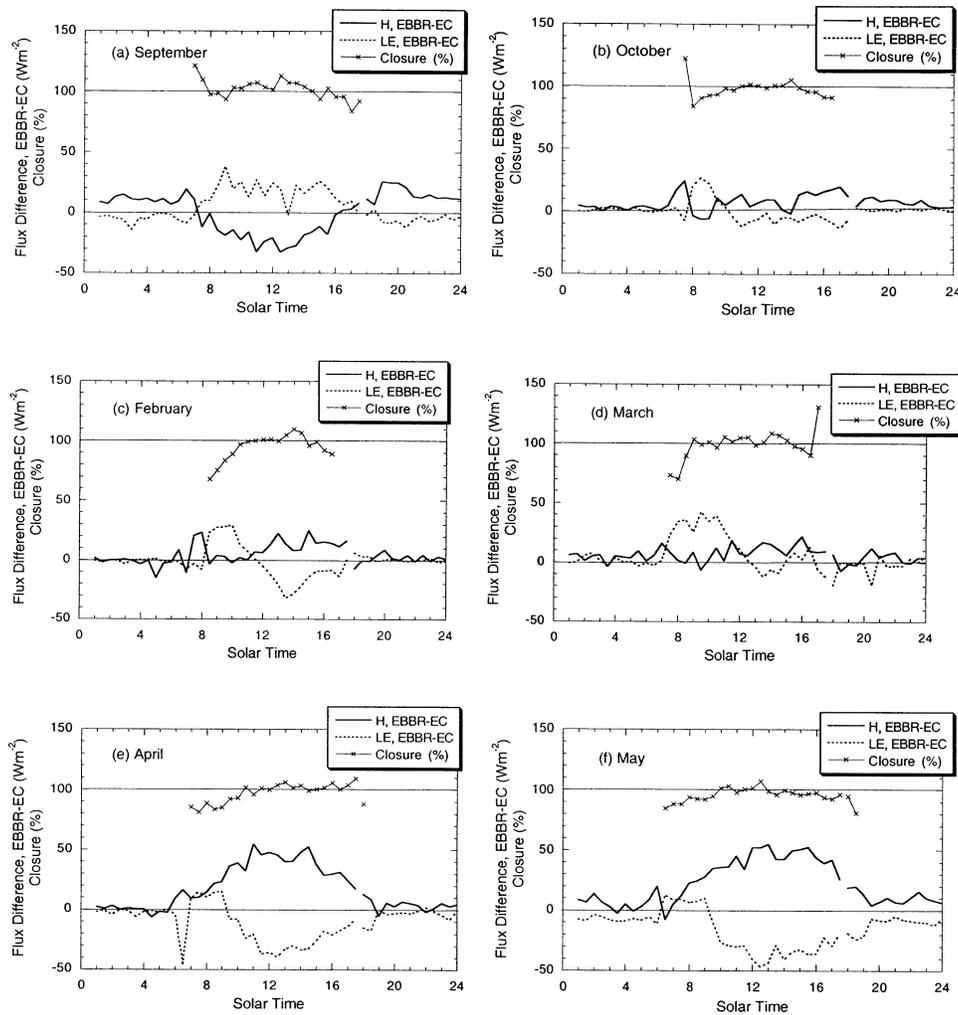
FIG. 11. The monthly mean diurnal cycle of EC closure in percent and EBBR minus EC differences in  $H$  and LE for six different months during 1 Sep 1999–31 May 2000. The EBBR estimates of flux used the available energy from the EC.
