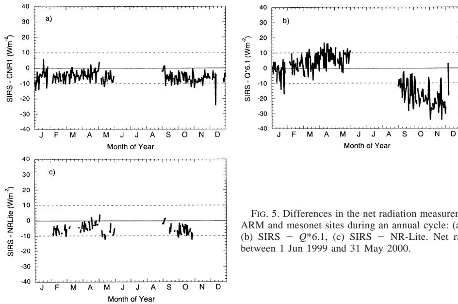
FIG. 5. Differences in the net radiation measurements between the ARM and mesonet sites during an annual cycle: (a)  $SIRS - CNR1$ , (b)  $SIRS - Q*6.1$ , (c)  $SIRS - NR-Lite$ . Net radiation collected between 1 Jun 1999 and 31 May 2000.
