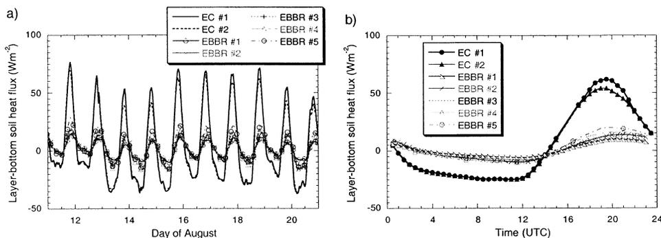
FIG. 16. (a) Time series and (b) 10-day diurnal average of the layer-bottom soil heat flux ( $\text{W m}^{-2}$ ) at 5-cm depth as measured by seven heat flux plates (two at EC site, five at BR site) during 11–20 Aug 1999.
