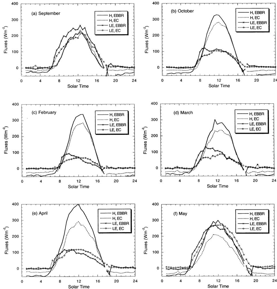
FIG. 10. Monthly mean diurnal cycle of sensible ( $H$ ) and latent heat flux ( $LE$ ) as estimated at the EBBR and EC sites at Foraker. The EBBR estimates of flux used the net radiation measured by the EC four-component SIRS for six different months during 1 Sep 1999–31 May 2000.
