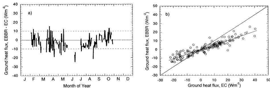
FIG. 6. (a) Differences in daily ground heat flux between the EBBR and EC sites during an annual cycle. (b) Scatterplot of BR vs EC daily totals of ground heat flux collected between 1 Jun 1999 and 31 May 2000.
