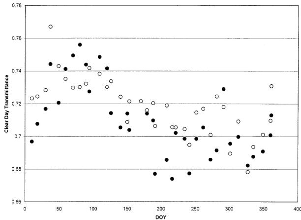
FIG. 1. Seasonal change of maximum measured 10-day period transmittance ( $T_{t,max}^{meas}$ , filled circles) and corresponding averaged 10-day period values of computed clear day transmittance ( $T_{t,max}$ , empty circles) as a function of day of year (DOY).
