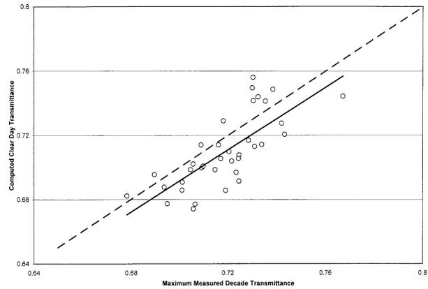
FIG. 2. Ten-day average of computed clear day transmittances ( $T_{t,max}$ ) as a function of corresponding maximum measured 10-day period transmittance ( $T_{t,max}^{meas}$ ). Solid line is the regression line and a 1:1 line (dashed) is included for reference. Statistics are presented in Table 1.
