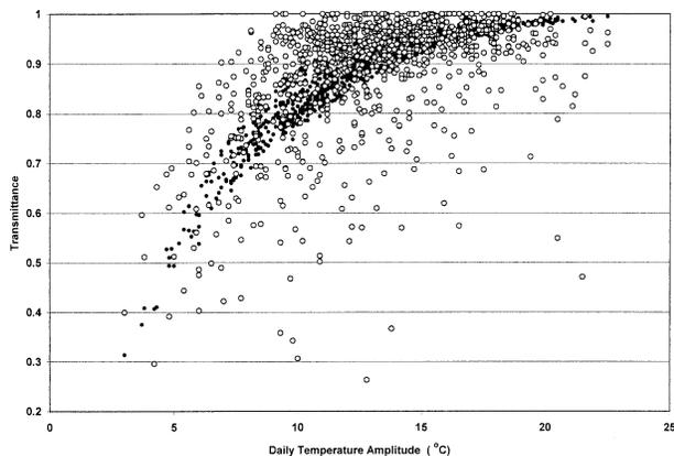
FIG. 3. Computed ( $T_{f,max}$ , empty circles) and measured ( $T_{f,max}^{meas}$ , filled circles) values of realized proportions of clear day transmittances plotted against the corresponding daily temperature ranges.
