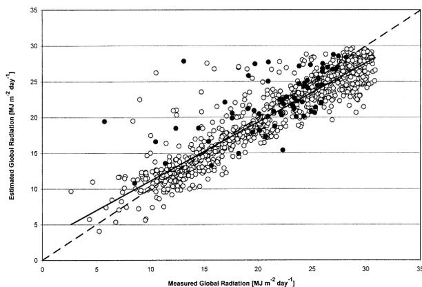
FIG. 4. Estimated global radiation ( $R_{gh}$ ) as a function of measured global radiation. Filled circles indicate days for which rainfall was recorded. Solid line is the regression line and a 1:1 line (dashed) included for reference. Statistics are presented in Table 1.
