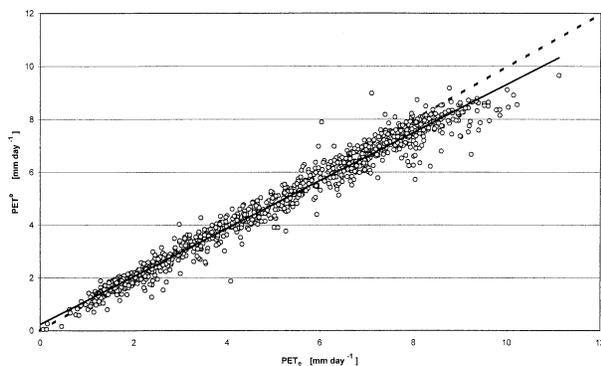
FIG. 7. Penman's PET computed using saturated vapor pressure at min daily temperature instead of measured daily averaged vapor pressure ( $PET_e$ ) as a function of  $PET_e$ . For details of computation see text. Solid line is the regression line and a 1:1 line (dashed) included for reference. Statistics are presented in Table 1.
