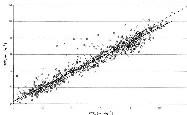
FIG. 6. Penman's PET computed using estimated global radiation ( $PET_e$ ) as a function of Penman's PET computed using measured global radiation ( $PET_m$ ). Solid line is the regression line and a 1:1 line (dashed) included for reference. Statistics are presented in Table 1.
