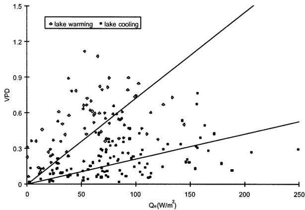
FIG. 6. Scattergram and regression lines illustrating the variation in VPD and  $Q_e$  for the periods when Skeeter Lake was warming and cooling.
