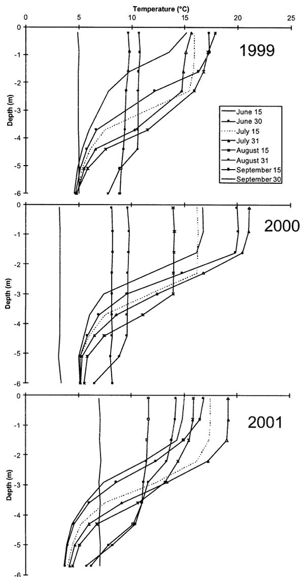
FIG. 3. Water temperature profiles from 1999 and 2000.
