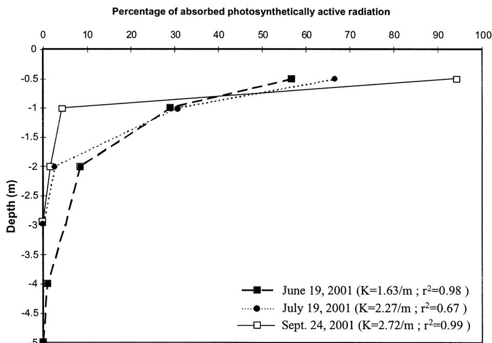
FIG. 2. Attenuation of radiation in Skeeter Lake for three selected days in 2001. The percentages of absorbed radiation are within each layer, bounded by measurements points above the lake surface and at 0.5-, 1-, 2-, 3-, 4-, and 5-m depths,  $K$  is the attenuation coefficient. The regression value between in (PAR) and water depth is also shown.
