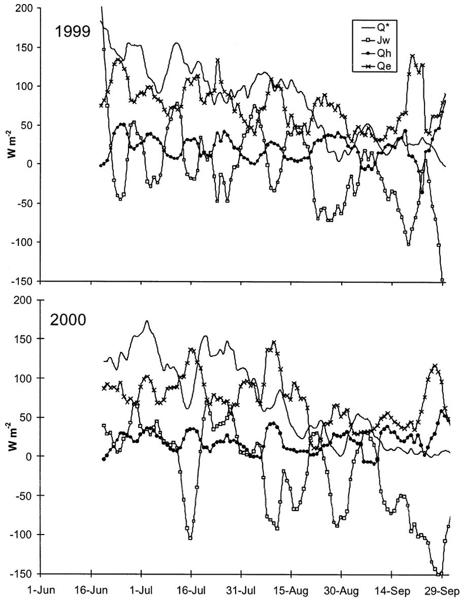
FIG. 5. The energy budget of Skeeter Lake in 1999 and 2000, beginning when the lake tower was deployed. Values presented are 5-day running means.
