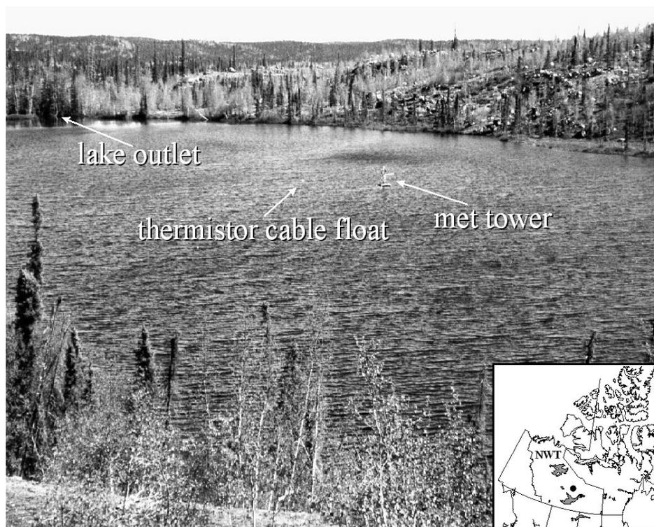
FIG. 1. Photo of Skeeter Lake looking east. The location of the tower, thermistor cable float, and lake outlet are identified. The measurements of surface inflow and rainfall were near the north shore immediately to the left of the photo.
