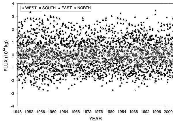
FIG. 3. Time series of the monthly means (kg) of the water vapor fluxes across the four main boundaries, west (diamond), east (triangle), south (square), and north (circle).
