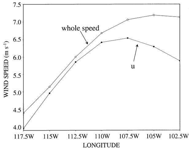
FIG. 6. The meridional average across the basin of the zonal wind component  $u$  ( $\text{m s}^{-1}$ ) and the complete wind speed (square root of  $u^2 + v^2$ , in  $\text{m s}^{-1}$ ) extracted from the 20-yr (1979–98) climatology of the 850-hPa wind field from the NCEP–NCAR reanalysis data.
