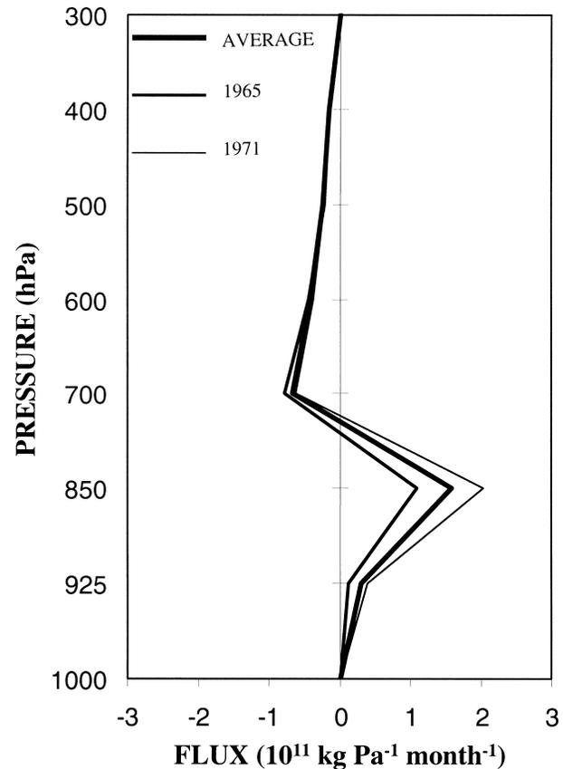
FIG. 12. Vertical profiles of the annual mean of the net moisture fluxes ( $\times 10^{11}$  kg Pa $^{-1}$  month $^{-1}$ ) for the driest year (1971; thin line), the wettest year (1965; thick line) during the 40-yr period (1962–2001), and the 40-yr period average (thickest line).
