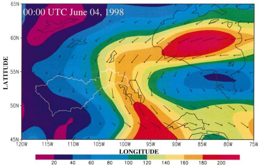
FIG. 8. An example in Jun 1998 showing that Hudson Bay is a moisture source for the Saskatchewan River basin. Plotted is the moisture transport vectors and their magnitude (color shaded, in  $\text{kg m}^{-1} \text{s}^{-1}$ ) at 0000 UTC 4 June 1998. Boundaries of the Saskatchewan River basin are shown in white.
