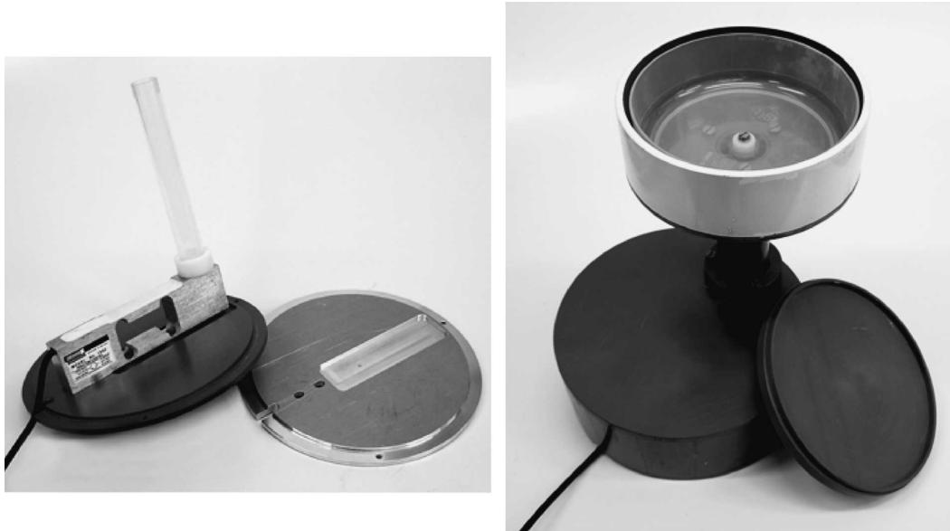
FIG. 2. (left) Load cell affixed to a PVC base plate. An aluminum base plate option is also shown (note the depression to allow the load cell to bend). (right) Microlysimeter showing the empty plastic sampling dish and protective cover for rain or storage.
