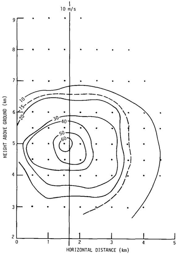
FIGURE 10.—Residence time of hailstones in the updraft model as a function of starting position. Growth rate is  $0.33 \text{ m}\cdot\text{s}^{-1}\cdot\text{min}^{-1}$ . Isoleths of elapsed time are labeled in min. Coordinates are as in figures 3 and 8.
