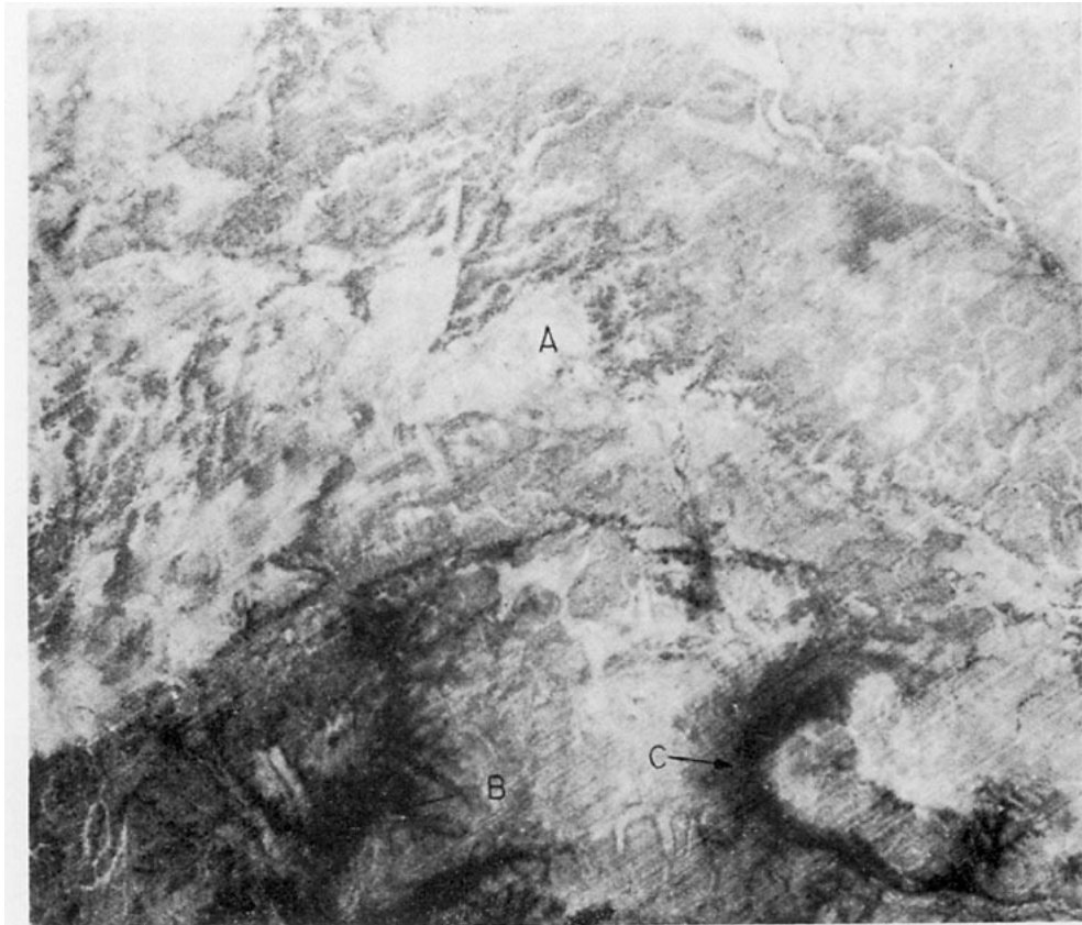
FIG. 4. Existence of winds in the Susitna and Copper River valleys on 21 January 1975 is indicated as dark bands in the IR imagery while Tanana Valley without wind remains cold and appears white. (A, B, and C denote Tanana, Susitna, and Copper River valleys).
