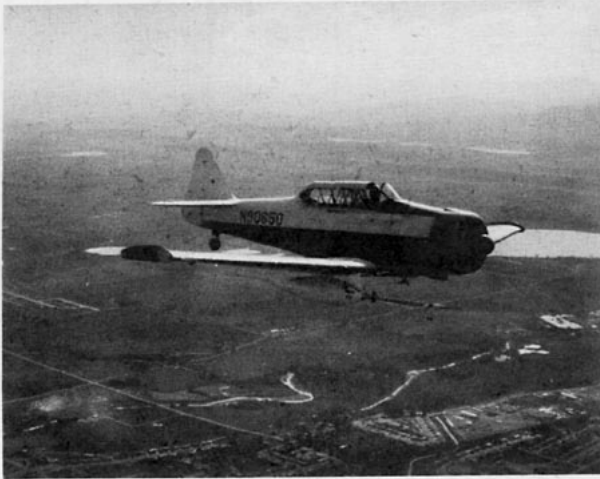
FIG 1. Subcloud severe storms measurement aircraft. The North American T-6 aircraft has been extensively modified to carry the AADS-2B system. The boom structure positions some of the sensing probes ahead of the aircraft to minimize fuselage-wing flow and pressure effects. The boom supports the Rosemount temperature sensor, pitot-static tube and the \alpha , \beta vane system. The \alpha and \beta vane units, along with the gyro-referenced platform, provide data on the vertical and lateral air motions near and within the severe storms. The vanes are constructed of lightweight balsawood and are internally mass balanced to improve the response characteristics. The boom is of aluminum-stainless steel construction and has a natural frequency of 11 Hz.
