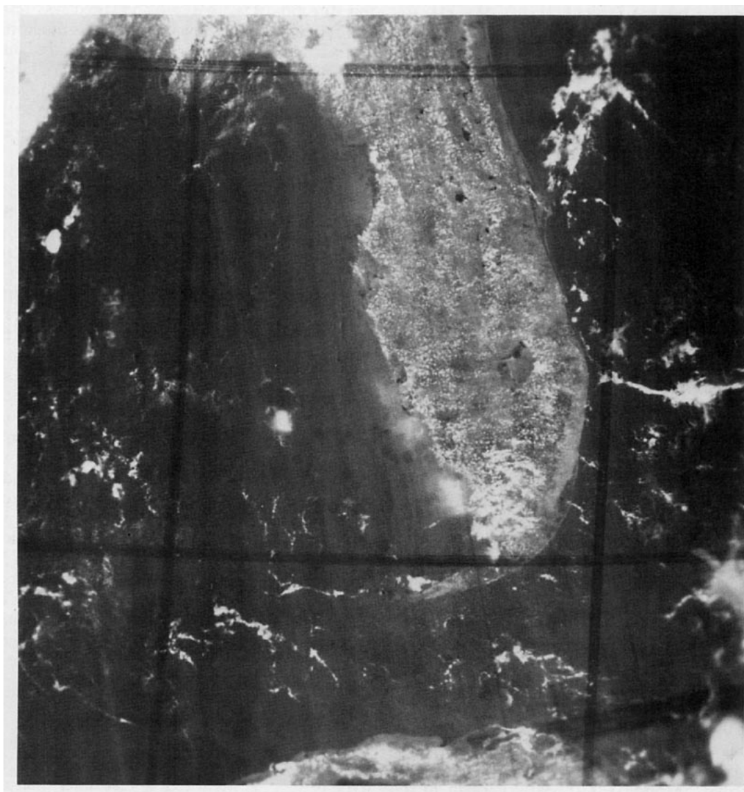
FIG. 5. DMSP visual (0.54 km resolution) enlargement of the Florida region at 1223 EST 6 June 1973. Calm seas are implied by brilliant sunglint reflection along the southwest coast.
