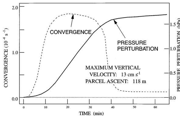
FIG. 11. Model-simulated surface pressure perturbation and estimated convergence versus time at the midpoint of cross section  $BB'$  shown in Fig. 8. The point  $t = 0$  corresponds to 0500 UTC 9 March 1992.
