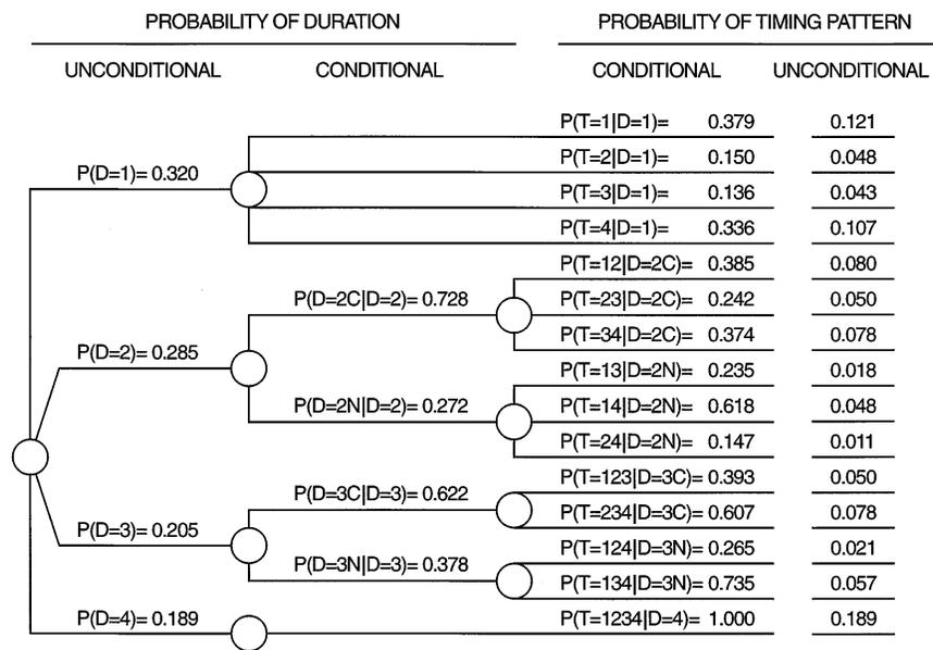
FIG. 3. Precipitation timing tree for a 24-h period divided into four 6-h subperiods; Monongahela Basin, March, from 1200 UTC.
