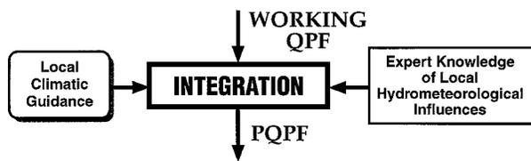
FIG. 8. Integration phase in a scheme for judgmental processing of information from multiple sources into the PQPF for a river basin.
