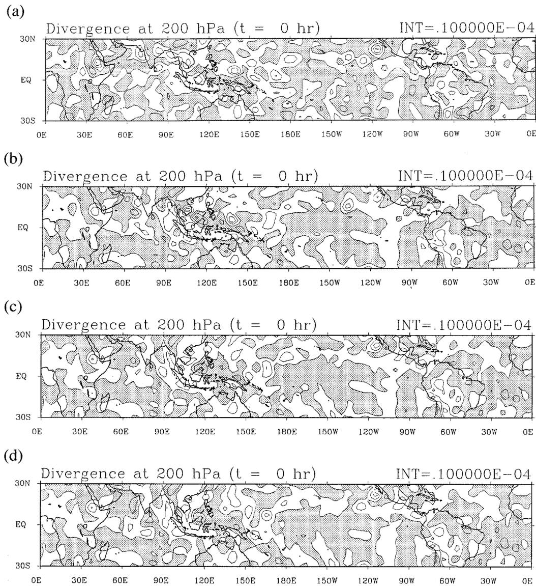
FIG. 13. Divergence at 200 hPa at the end of assimilation window for (a) the initial guess, (b) NOMP, (c) MP, and (d) MP+RR. Contour interval is  $1 \times 10^{-5} \text{ s}^{-1}$ . Negative areas are shaded.
