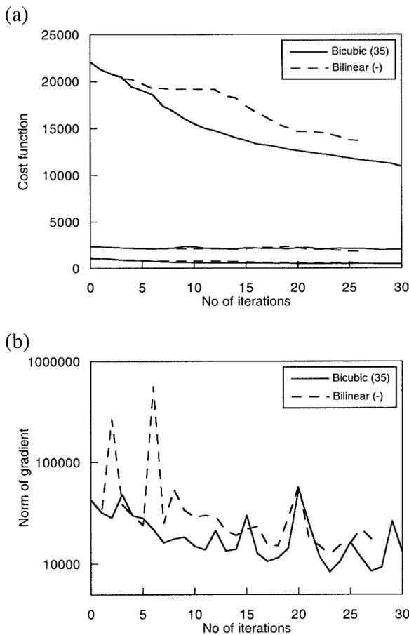
FIG. 8. Same as Fig 6, except for MP+RR with bicubic and bilinear interpolations for precipitation data. In (a) the upper two lines are the discrepancy terms for radiosonde and pibal data, the middle two lines are the penalty terms, and the lower two lines are the discrepancy terms for precipitation data.
