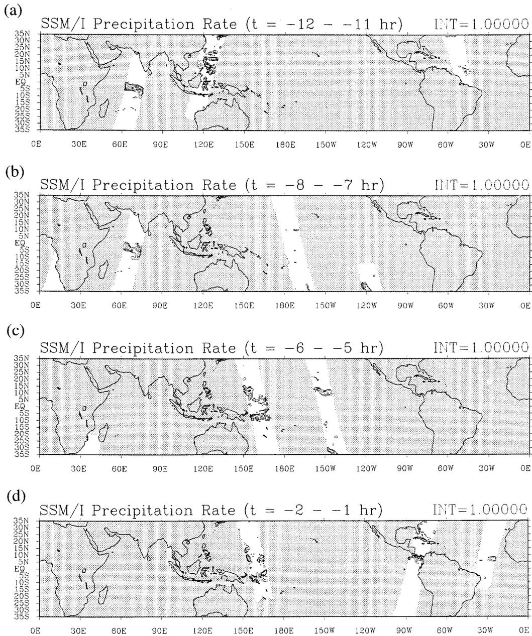
FIG. 2. SSM/I precipitation rates for (a) 0000–0100, (b) 0400–0500, (c) 0600–0700, and (d) 1000–1100 UTC 22 August 1992. Contour intervals are 0.25, 0.5, 1, 2, and 4 mm h<sup>-1</sup>. Data-void areas are shaded.
