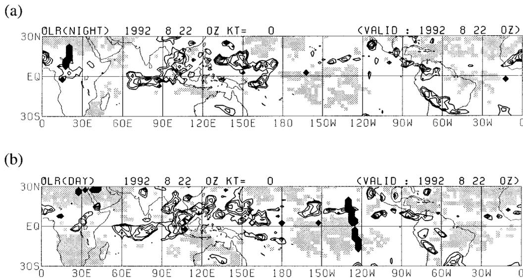
FIG. 4. Composites of outgoing longwave radiation for (a) night pass and (b) day pass of NOAA satellites for 22 August 1992. Contour interval is  $25 \text{ W m}^{-2}$  and contours greater than  $200 \text{ W m}^{-2}$  are omitted. Areas of greater than  $275 \text{ W m}^{-2}$  are lightly shaded. Data-void areas are densely shaded.
