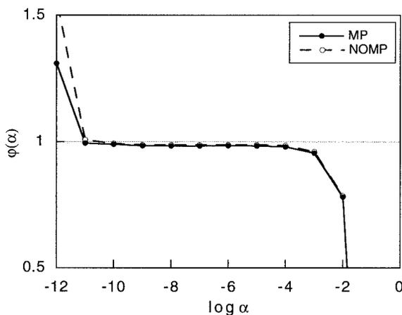
FIG. 5. Variations of the function  $\varphi(\alpha)$  with  $\log \alpha$  for NOMP and MP with  $r = 8 \times 10^{20} \text{ s}^4$ . The initial guess is taken as  $x_0$ .
