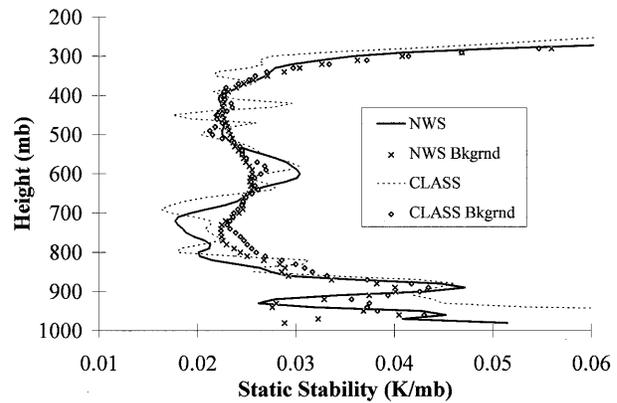
FIG. 12. Composite static stability profiles calculated from composite potential temperature profiles, using soundings with layers that have  $p_{max}$  between 600 and 700 mb. Also shown are the composites based on using all NWS and CLASS soundings analyzed here.
