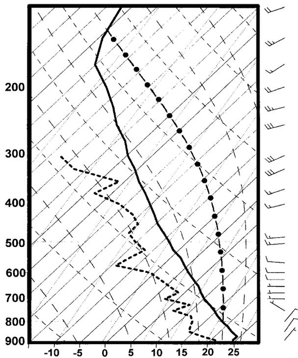
FIG. 3. Skew  $T$ - $\log p$  diagram representing the temperature (solid line), moisture (dashed line), and wind profile over Rapid City at the time of the storm (0500 UTC 6 July). Horizontal axis is temperature ( $^{\circ}\text{C}$ ); vertical axis is pressure (mb). The wind is given along the right edge, with a full barb representing  $10\text{ m s}^{-1}$ . The 0000 UTC Rapid City sounding was modified with (0500 UTC) surface data and VAD wind profile data from the KUDX radar for this figure.
