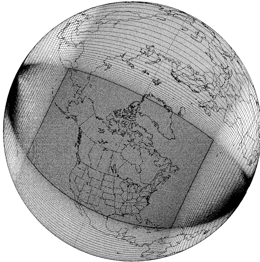
FIG. 1a. The 255 \times 289 variable-resolution horizontal grid of the currently operational regional configuration of the GEM model: it has uniform 0.33^\circ resolution over the 59.07^\circ \times 77.22^\circ ( 180 \times 235 ) central window.
