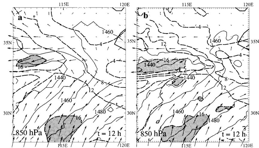
FIG. 19. Simulated 850-mb geopotential height (thin solid lines every 10 gpm), wind speed (thick dashed lines every 4  $\text{m s}^{-1}$ ), and wind vectors from the Kain-Fritsch experiments at (a) 54 km and (b) 18 km. Areas with wind speed exceeding 16  $\text{m s}^{-1}$  are shaded.
