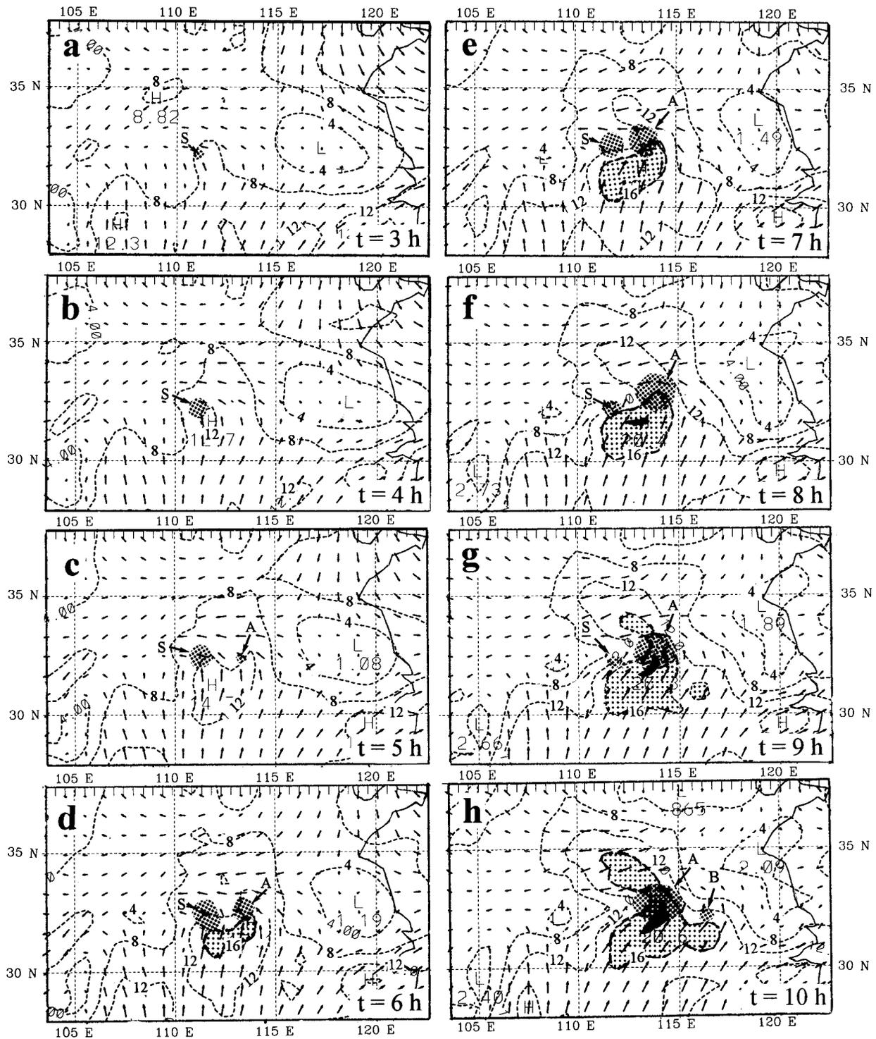
FIG. 13. Simulated 850-hPa wind vectors and speeds (dashed lines every 4 m s<sup>-1</sup>) every hour from  $t = 3$  h (0300 UTC 12 June) to  $t = 10$  h (1000 UTC 12 June). Heavy-stippled areas depict rainstorms S and A, and light-stippled and black areas indicate the wind speeds greater than 16 and 20 m s<sup>-1</sup>, respectively.
