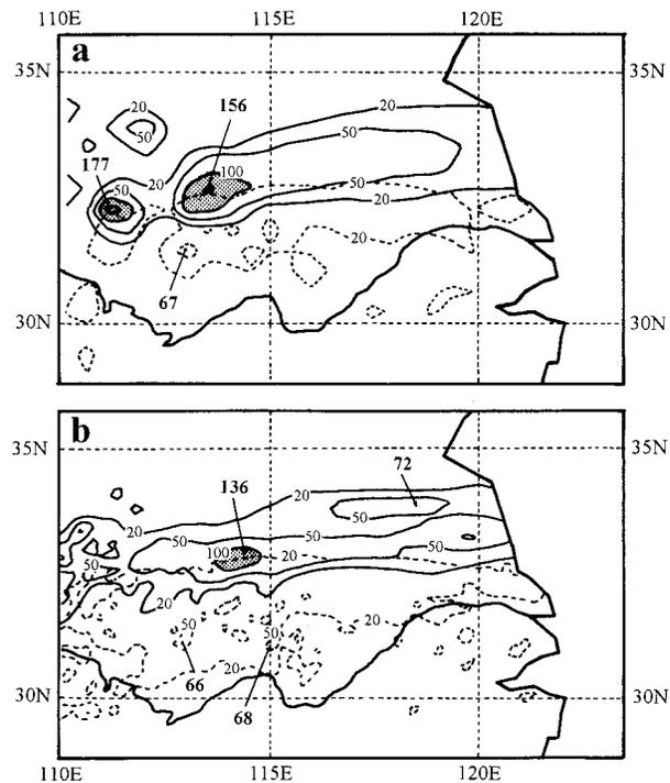
FIG. 18. Simulated 24-h rainfall produced in experiments using the Kain–Fritsch cumulus scheme (dashed) and explicit scheme (solid) from (a) the 54-km experiment (KF54) and (b) the 18-km experiment (KF18). Areas with rainfall exceeding 100 mm are shaded.
