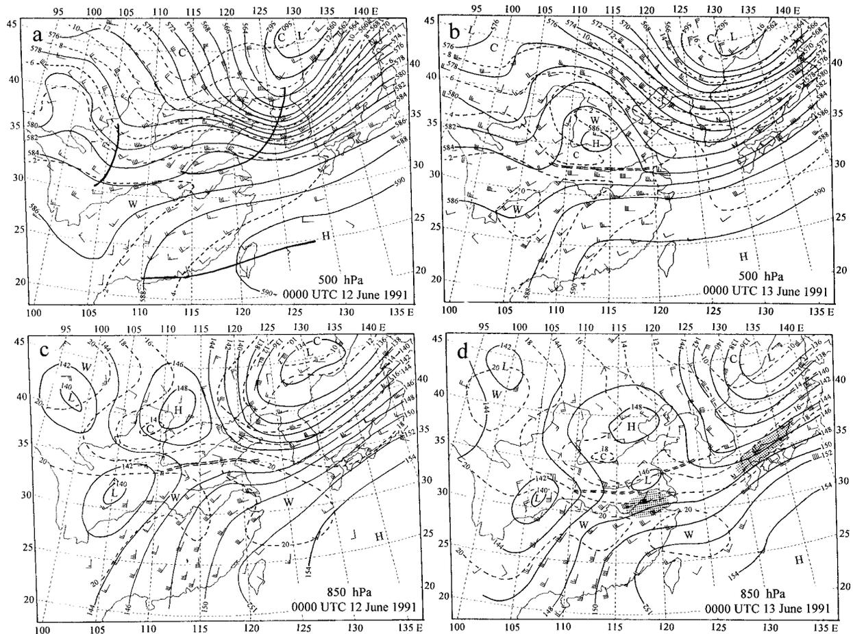
FIG. 3. Manual analyses of the geopotential height (every 20 gpm) and temperature (every 2°C) fields at (a) 500 hPa, 0000 UTC 12 June 1991; (b) 500 hPa, 0000 UTC 13 June 1991; (c) 850 hPa, 0000 UTC 12 June 1991; and (d) 850 hPa, 0000 UTC 13 June 1991. Thick solid lines depict trough lines and the ridge line (WPSH), double dashed lines represent shear lines. Observed winds are plotted. Areas of wind speeds over  $16 \text{ m s}^{-1}$  are shaded in (d) to verify the model results shown in Fig. 7.
