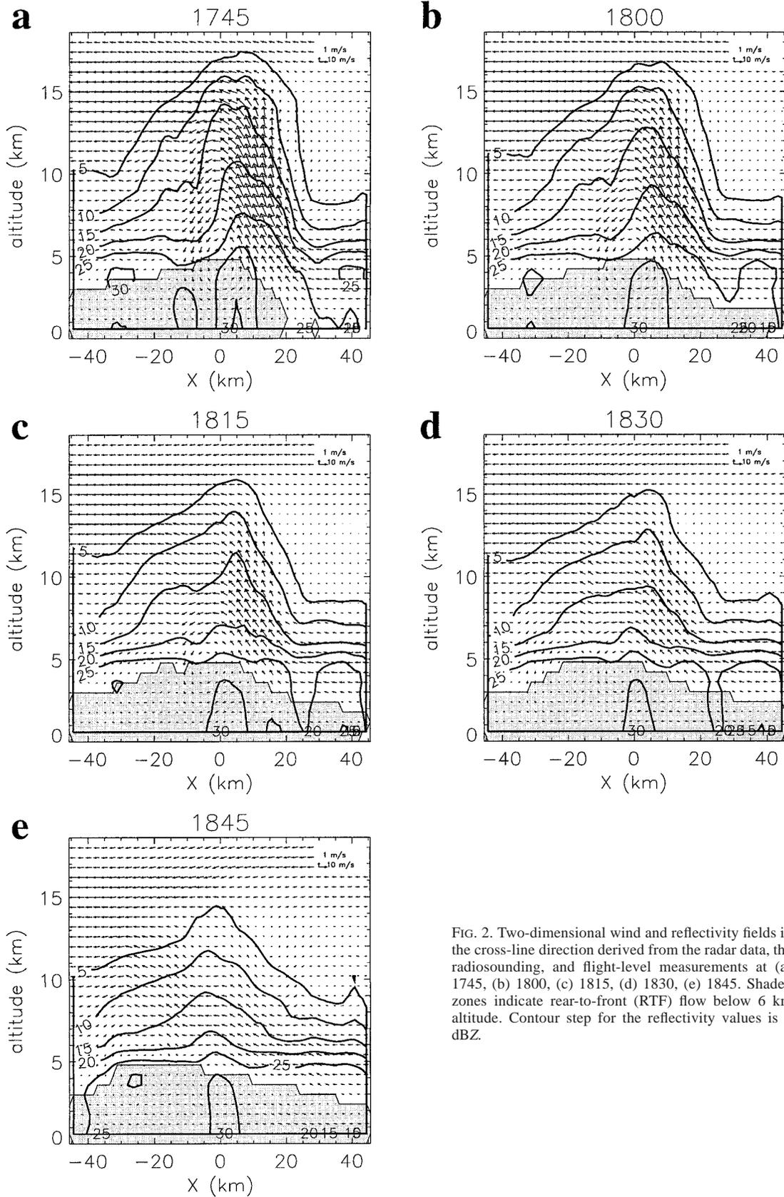
FIG. 2. Two-dimensional wind and reflectivity fields in the cross-line direction derived from the radar data, the radiosounding, and flight-level measurements at (a) 1745, (b) 1800, (c) 1815, (d) 1830, (e) 1845. Shaded zones indicate rear-to-front (RTF) flow below 6 km altitude. Contour step for the reflectivity values is 5 dBZ.
