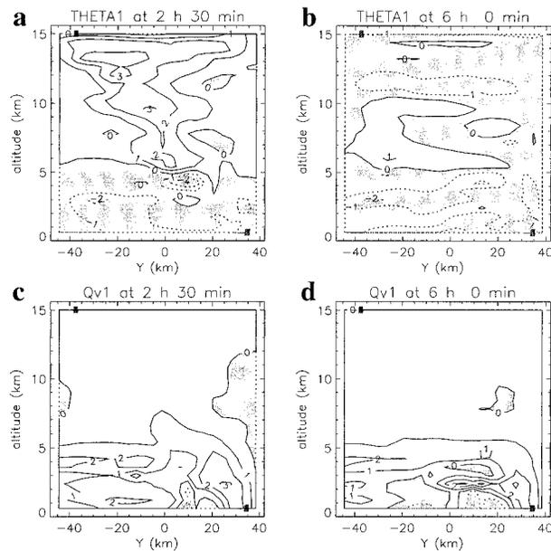
FIG. 9. Potential temperature perturbations (in K) at (a) 2 h 30 min, (b) 6 h, and water vapor perturbations (in  $\text{g kg}^{-1}$ ) at (c) 2 h 30 min, (d) 6 h, for the CONTROL run.
