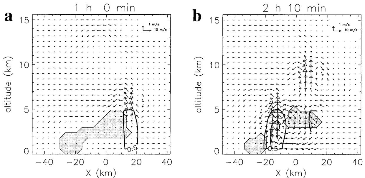
FIG. 4. Wind and total precipitation (rain + snow + graupel) fields for the QVSAT run at (a) 1 h and (b) 2 h 10 min of simulation time. Shaded zones indicate low-level (below 6-km altitude) RTF flow. Contour step for the precipitation content is  $1 \text{ g kg}^{-1}$ , starting from  $0.5 \text{ g kg}^{-1}$ .
