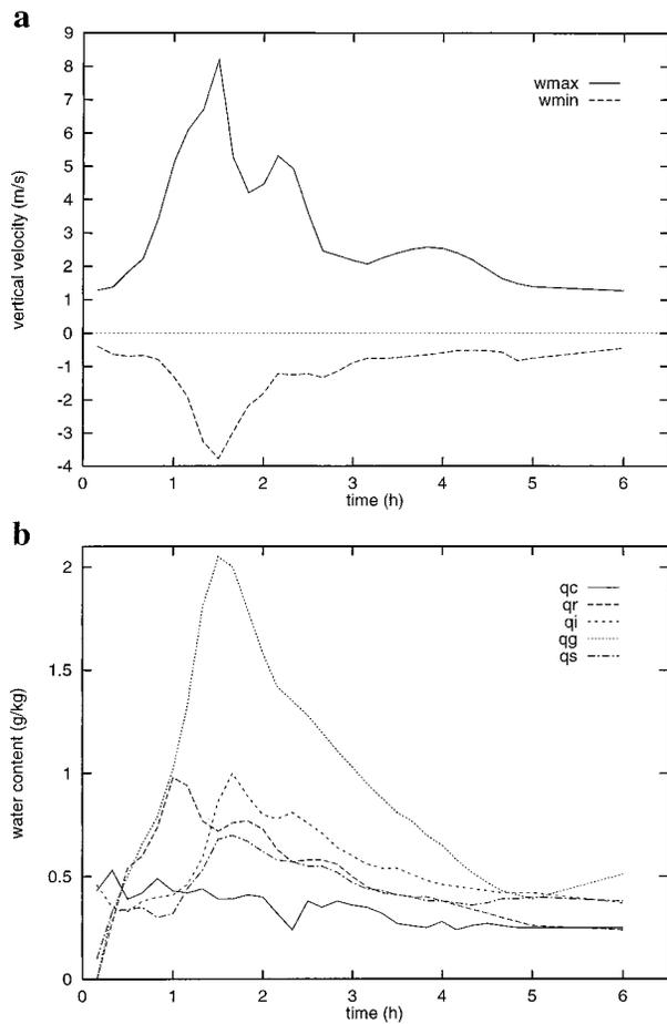
FIG. 7. Evolution of (a) the maximum and minimum vertical velocities, (b) the average of the different water contents over the area where hydrometeors are present, for CONTROL run.
