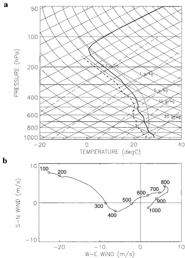
FIG. 1. Composite sounding based on the radiosonde launched from R/V *Shiyun 3* at 1700 and P3 N43RF flight-level measurements (a) skew  $T$ - $\log p$  diagram, (b) wind hodograph (the different levels are indicated in hPa).
