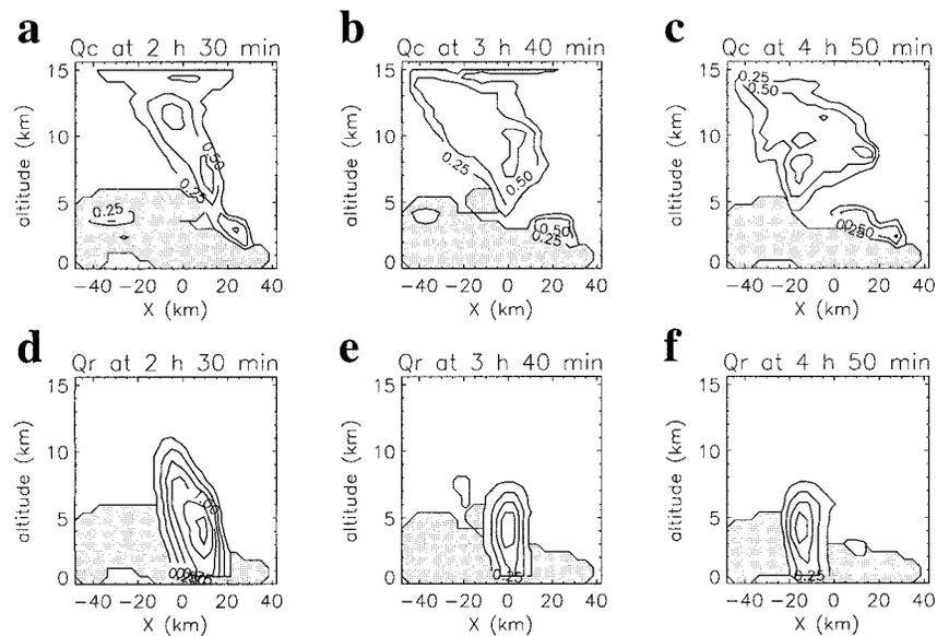
FIG. 11. Microphysical fields for the NOICE run: cloud water mixing ratio  $q_c$  at (a) 2 h 30 min, (b) 3 h 40 min, (c) 4 h 50 min; rain mixing ratio  $q_r$  at (d) 2 h 30 min, (e) 3 h 40 min, (f) 4 h 50 min. Shaded zones indicate low-level (below 6-km altitude) RTF flow. Contour step is  $0.25 \text{ g kg}^{-1}$ .
