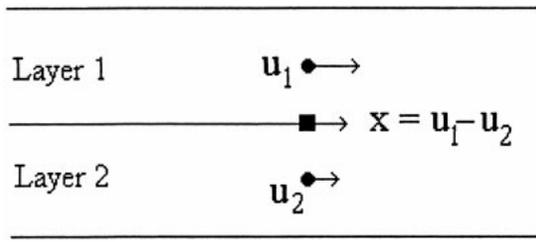
FIG. 1. A schematic of a two-layer diffusive model. Here,  $u_1$  ( $u_2$ ) is the velocity in the Layer 1 (Layer 2) and  $x$  is the vertical shear.
