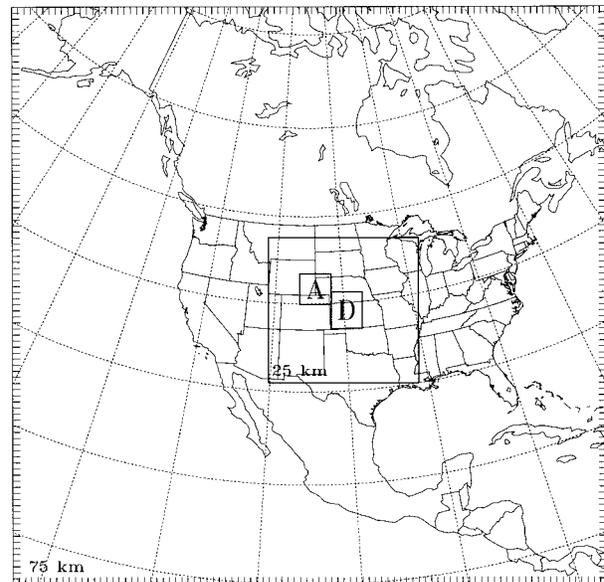
FIG. 1. Domain configurations of the MM5 simulations. The letters A and D mark the areas that are evaluated for sensitivities to various forecast aspects using the adjoint model.
