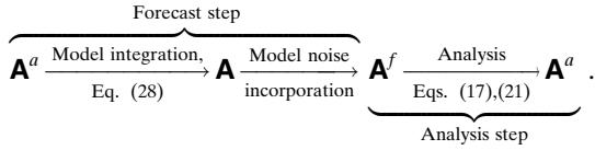
Although the first  $\mathbf{A}^a$  of the diagram is associated with the time step before that of  $\mathbf{A}$ ,  $\mathbf{A}^f$ , and the latter  $\mathbf{A}^a$ , this ambiguity becomes moot by focusing on the analysis step and the forecast step separately.
