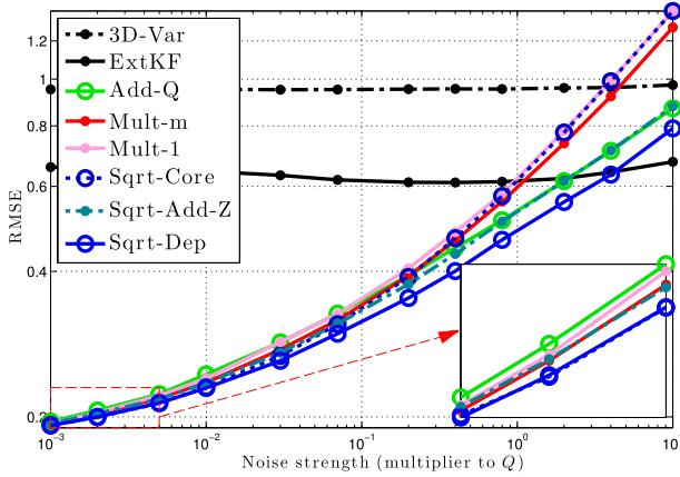
FIG. 5. Performance benchmarks as a function of the noise strength, obtained with the Lorenz-96 model and  $N = 25$ . Both axes are logarithmic. On average, when  $\mathbf{Q}$  is multiplied by  $10^{-3}$  ( $10^{-2}$ ,  $10^{-1}$ ,  $10^0$ ,  $10^1$ , respectively), the model noise makes up approximately 0.5% (4%, 20%, 70%, 90%, respectively) of the growth in the spread of the ensemble between each assimilation. The climatology averages an RMSE score of approximately 4.
