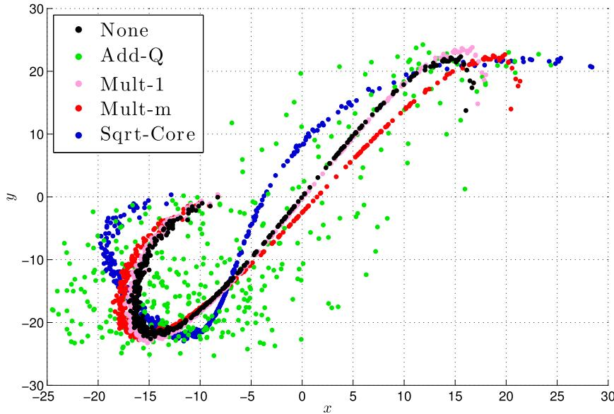
FIG. 1. Scatterplot of ensemble forecasts with the three-dimensional Lorenz-63 system (Lorenz 1963) using different schemes to account for the model noise, which is specified by  $\Delta t Q = \text{diag}([36.00, 3.60, 1.08])$  and makes up approximately 30% of the total spread of the updated ensembles. Each dot corresponds to the “(x, y)” coordinate of one realization among  $N = 400$ .
