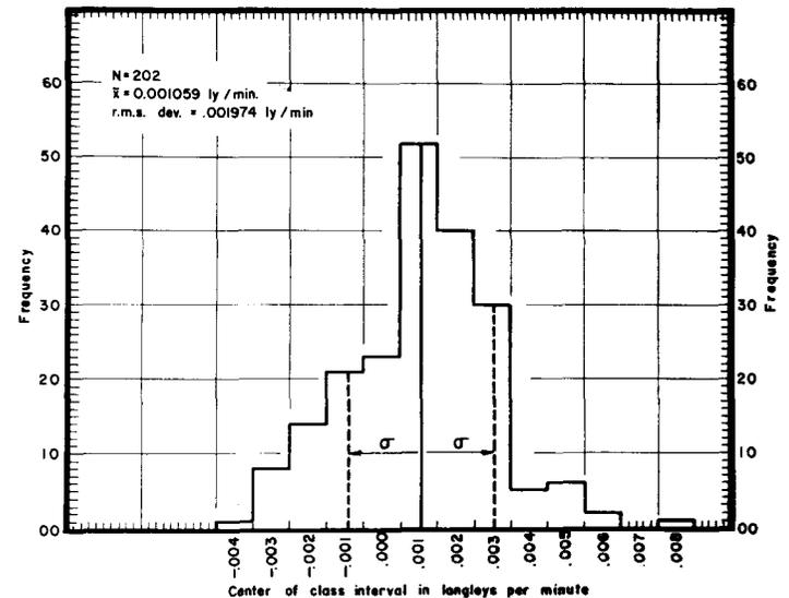
FIGURE 1.—Frequency distribution of the difference in net radiation observed with airborne economical radiometer (radiometersonde) and the Suomi ventilated radiometer.
