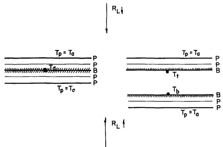
FIGURE 2.—Cross section of the disc airborne economical radiometer (left) and standard airborne economical radiometer (right). Cross hatching indicates blackened aluminum sensing surface;  $R_L$  is infrared radiation current; black dots are temperature sensors; subscripted T's refer to polyethylene, air, top, and bottom temperatures; upper case P's to polyethylene ventilation shields.
