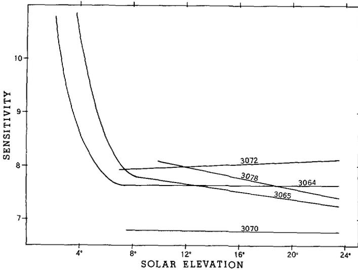
FIGURE 2.—Variation of pyranometer sensitivity (mv/(ly. min.<sup>-1</sup>)) with solar elevation from Amundsen-Scott (South Pole) direct solar calibrations.
