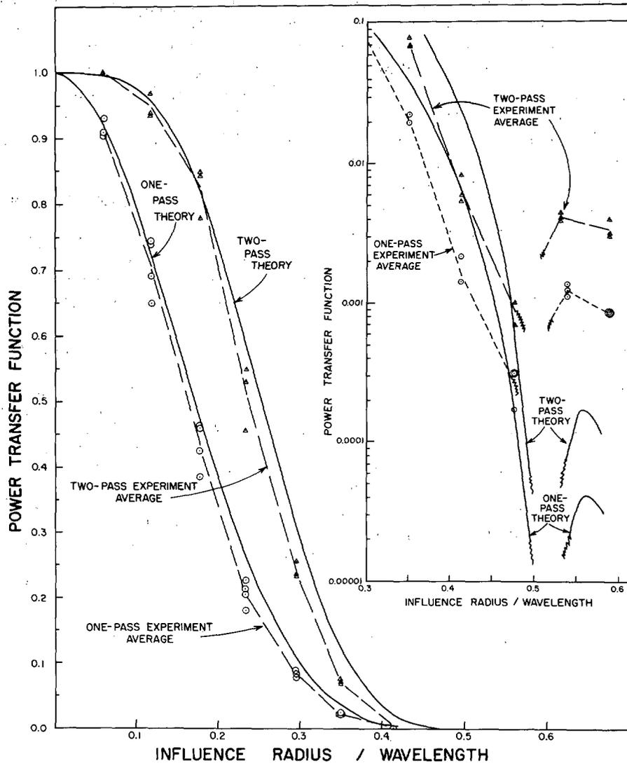
FIGURE 2.—Power transfer functions for one- and two-pass applications of the method of successive corrections with a zero guess field for  $(R/d)=1.75$  and  $d=\Delta x$ .
