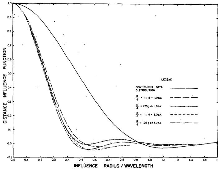
FIGURE 1.—Distance influence function for various influence radii and data separations as a function of the ratio of influence radius to wavelength.
