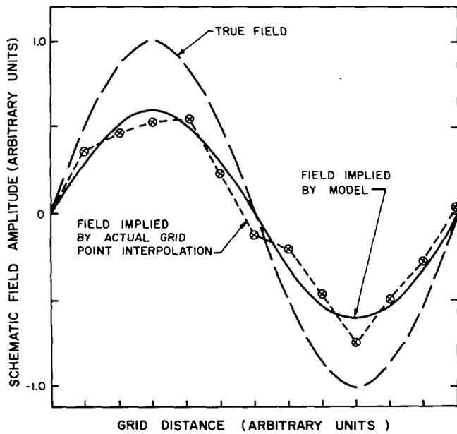
FIGURE 3.—Schematic illustration of the difference between the model and actual interpolations.
