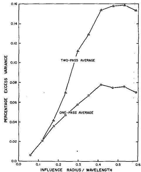
FIGURE 4.—Percentage excess variance for one- and two-pass applications of the method of successive corrections with a zero guess field for  $(R/d)=1.75$  and  $d=\Delta x$ .
