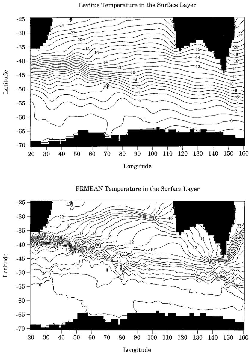
FIG. 1. Sea surface temperature, contoured in  $1^{\circ}\text{C}$  intervals. (a) Levitus (1982) annual mean climatology; note the slope of the isotherms west of Australia indicating the southward flowing Leeuwin Current. (b) FRAM mean SST; note the difference in the slope of the isotherms west of Australia against (a). (c) The difference (a) - (b). Dark shaded areas indicate FRAM heat flux into the ocean.
