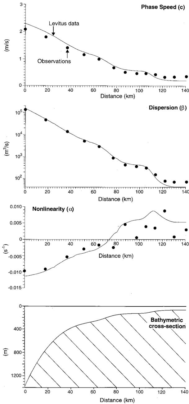
FIG. 5. Coefficients of the K-dV equation calculated from CTD data of 1995 (points) and from Levitus climatic data (solid line) as a function of distance across the shelf-break region. The bathymetric cross section is also shown.
