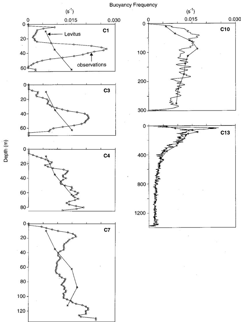
FIG. 4. Vertical profiles of the Brunt-Väisälä frequency calculated from CTD data of 1995 at locations C1, C3, C4, C7, C10, and C13 and calculated from Levitus climatic data.
