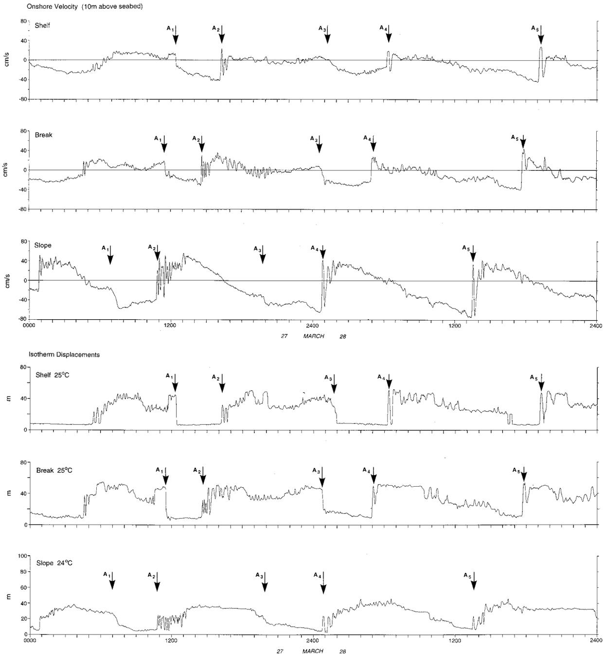
FIG. 3a. Time series of onshore velocity component measured 10 m above the seabed and isotherm displacements from the slope, break and shelf locations over the period 0000 27 to 2400 28 March 1992.
