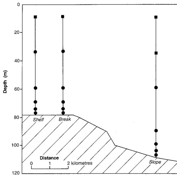
FIG. 2. Bathymetric cross section showing mooring locations and current meter positions for the 1992 dataset. Current meters were Steedman Acoustic current meters (●) or InterOcean S4 electromagnetic current meters (■).
