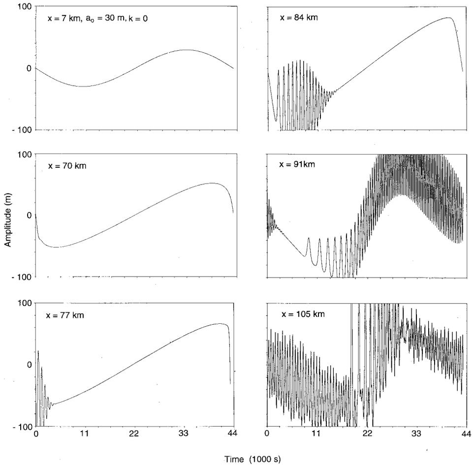
FIG. 10. Numerical results from the generalized K-dV equation. The waveform over one period is shown at different distances ( $x$ ) from the origin. Calculations are for data from 1995. Initial amplitude 30 m,  $k = 0$ .
