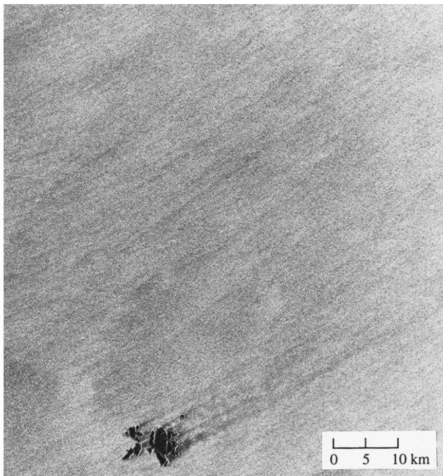
FIG. 1. ERS-1 SAR image of the sea surface over Bass Strait ( 39^{\circ}09'S , 147^{\circ}20'E ) on 11 Aug 1992, with U_{10} = 17.6 \text{ m s}^{-1} and the wind from 245^{\circ} . The longitudinal striations on the sea surface are aligned approximately in the wind direction. The darkened areas associated with sheltered flow in the lee of the small islands indicate that the dark striations in the image are regions of reduced mean surface wind speed.
