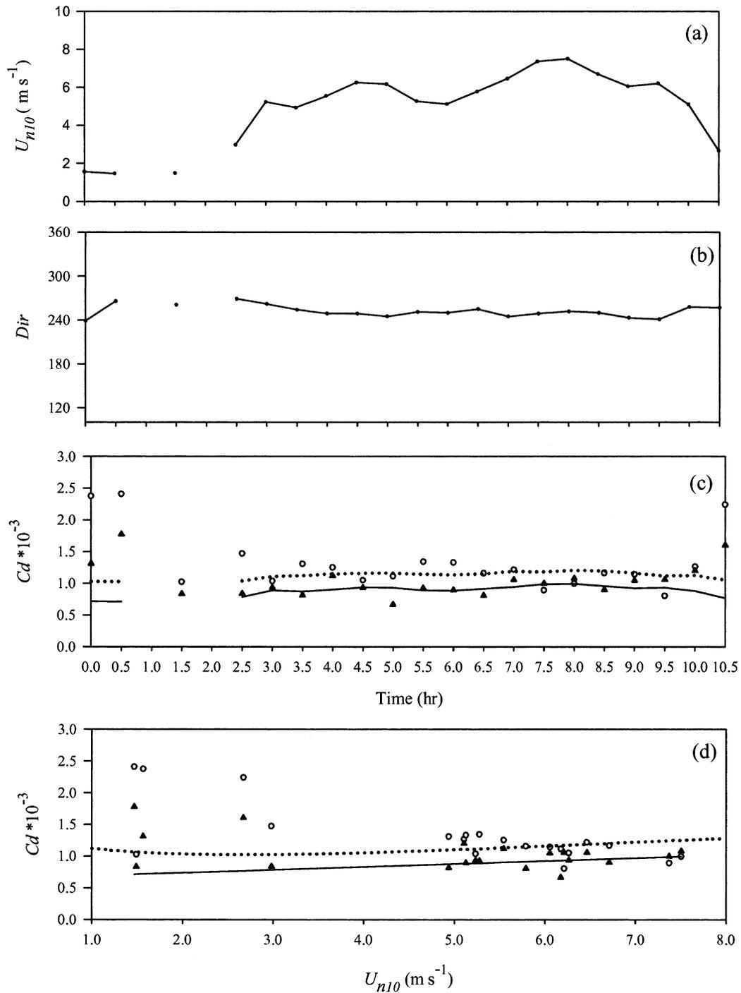
FIG. 8. An 11-h time series of (a) neutral wind speed, (b) wind direction, and (c) the drag coefficients. The  $C_d$  in (c) was calculated from flux measurements (open circles), from linear regression in Eq. (18) (solid lines), from the regression with wave age in Eq. (9) (solid triangles), and from Eq. (17) (dotted line). These  $C_d$  are plotted against the mean wind speeds  $U_{n10}$  in (d).
