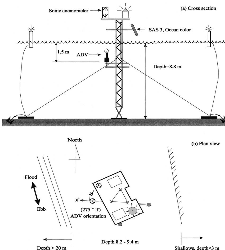
FIG. 2. Layout of the temporary fixed tower for the experiment: (a) cross section and (b) plan view.
