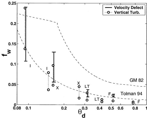
FIG. 2. Friction factors estimated using the velocity defect relation (solid vertical bars: QB95 only) and turbulence intensity (dashed vertical bars: both SD97 and QB95). Shown for comparison are the predictions from Tolman (1994) and Grant and Madsen (1982).
