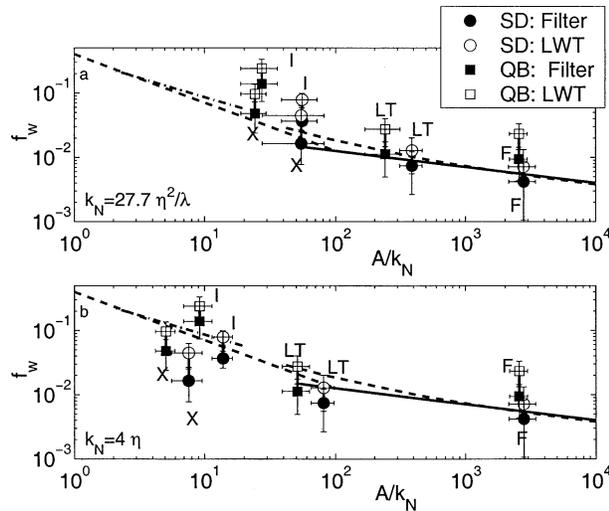
FIG. 5. Ensemble-averaged friction factors for the QB95 and SD97 experiments as a function of relative roughness,  $A/k_N$ . Symbols represent measured values for the linear wave theory method (open) and filter method (solid), a circle indicates SD97 data and a square QB95 data: (a)  $k_N = 27.7 \eta^2/\lambda$  and (b)  $k_N = 4\eta$ . For flat bed,  $k_N = 2d_{50}$ . Error bars are 5 times the standard error. Lines are as in Fig. 4.
