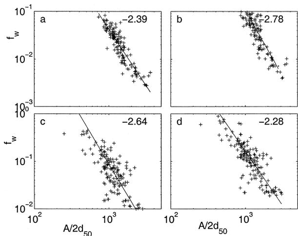
FIG. 10. Measured friction factors as a function of  $A/2d_{50}$ ; SD97 results are shown for (a) the filter method and for (b) the linear wave theory method. Corresponding QB95 results are shown in (c) and (d).
