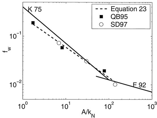
FIG. 8. Friction factors based on Eq. (23a), along with measurements. Also indicated are the smooth-turbulent regime from Fredsoe and Deigaard (1992) and the small  $A/k_N$  approximation from Kamphuis (1975).
