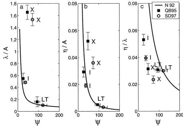
FIG. 1. Ensemble-averaged bedform dimensions for two field experiments compared with predictions by Nielsen [1992, Eqs. (3.4.3) and (3.4.8)]: (a) bedform wavelength  $\lambda$ , normalized by  $A$ , the significant wave semiexcursion as a function of the mobility numbers  $\psi$ ; (b) normalized bedform height,  $\eta/A$ ; and (c) bedform slope. Symbol indicators are I: irregular ripples, X: cross ripples, and LT: linear transition ripples. Error bars represent twice the standard error.
