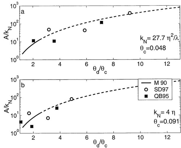
FIG. 6. Relative roughness,  $A/k_N$ , vs the normalized grain roughness Shields parameter,  $\theta_d/\theta_c$ . (a) Relative roughness estimated by  $27.7\eta^2/\lambda$  for data from QB95 (circles) and SD97 (squares). (b) Relative roughness estimated by  $4\eta$ . Also shown are the estimates from Madsen et al. (1990), originally obtained for  $\theta_d/\theta_c < 3$  (solid) and extrapolated here (dashed).
