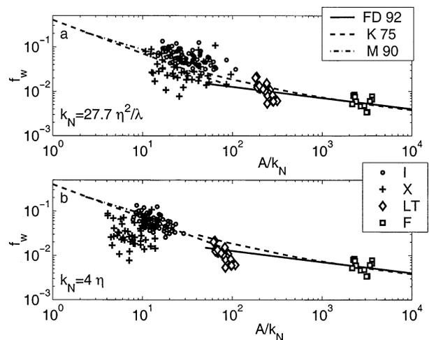
FIG. 4. Friction factors for the SD97 experiment as a function of relative roughness,  $A/k_N$  using two  $k_N$  estimators: (a)  $k_N = 27.7 \eta^2 / \lambda$  and (b)  $k_N = 4 \eta$ . For flat bed,  $k_N = 2d_{50}$ . Previous results are also shown, FD 92: Fredsoe and Deigaard (1992); K 75: Kamphuis (1975) general form and small  $A/k_N$  approximation; and M 90: Madsen et al. (1990).
