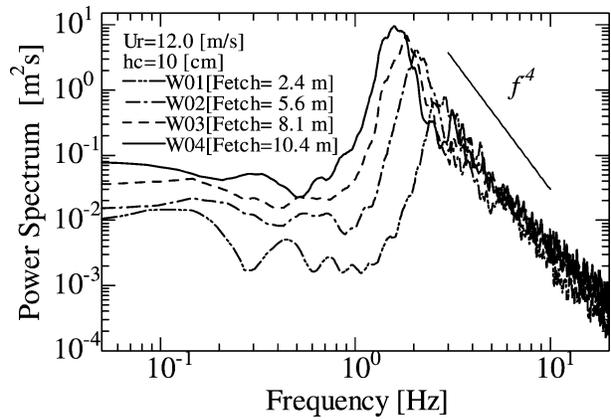
FIG. 4. Relationship of wave spectra  $S_\eta$  and fetch in the case of  $U_r = 12.0 \text{ m s}^{-1}$ .
