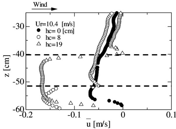
FIG. 9. Comparison of the vertical distribution of horizontal mean velocity  $\bar{u}$  at wind speed  $U_r = 10.4 \text{ m s}^{-1}$  among wind-wave tanks with duct heights of  $h_c = 0, 8.0,$  and  $19.0 \text{ cm}$ .
