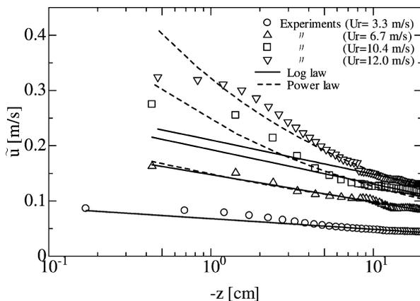
FIG. 13. Comparison of the vertical distribution of  $\tilde{u}$  near the water surface between the curves of the power and logarithmic laws at the respective wind speeds  $U_r$ .
