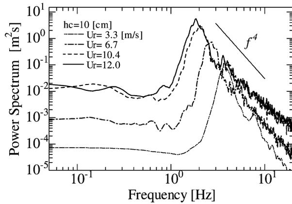
FIG. 3. Relationship between wave spectra  $S_\eta$  at the location of W03 and wind speeds  $U_r$  from 3.3 to 12.0  $\text{m s}^{-1}$ .
