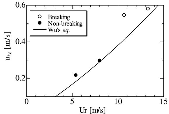
FIG. 5. Relationship between the air-side friction velocity  $u_{*a}$  and the reference wind speed  $U_r$ .
