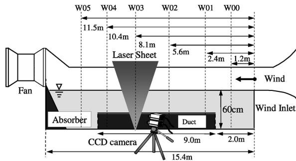
FIG. 1. Wind-wave tank with double bottom and measuring locations.
