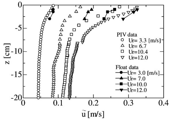
FIG. 11. Comparison of the vertical distribution of the mean velocity between pure wind-driven currents  $\tilde{u}$  measured using PIV and surface drift currents  $U_s$  measured by tracking floats.
