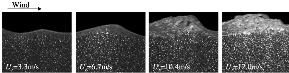
FIG. 2. Spatial water surface at the location of W03 affected by the wind with speed  $U_r$  from 3.3 to 12.0  $\text{m s}^{-1}$ .
