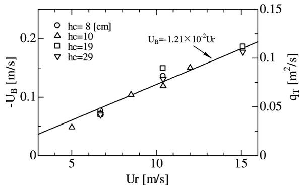
FIG. 10. Relationship among the mean velocity  $U_B$  of return flow (coordinate on the left), the wind speeds  $U_r$ , and the total mass flux  $q_T$  of the wind-driven currents (coordinate on the right) to  $U_r$ .
