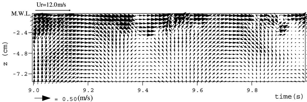
FIG. 6. Temporal variation of vertical distribution of the velocity vectors analyzed by the Direct-CCM below the mean water level at the location W03.
