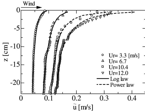
FIG. 15. Vertical distribution of the horizontal mean velocity  $\tilde{u}$  of wind-driven currents formulated by the logarithmic and power laws at respective wind speeds  $U_r$ .
