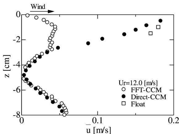
FIG. 7. Comparison of the vertical distribution of horizontal mean velocity  $\bar{u}$  among the Direct-CCM, the FFT-CCM, and the tracking floats at wind speed  $U_r = 12.0 \text{ m s}^{-1}$ .
