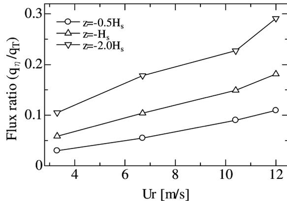
FIG. 12. Relationship between the ratio  $q_\eta/q_T$  (mass flux in the surface layer and total mass flux) and wind speed  $U_r$ .
