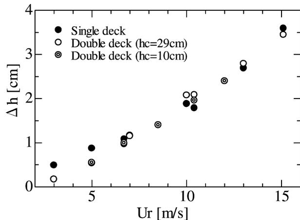
FIG. 8. Relationship of the reference wind speed  $U_r$  and the difference  $\Delta h$  between the mean water level at the locations of W00 and W05.
