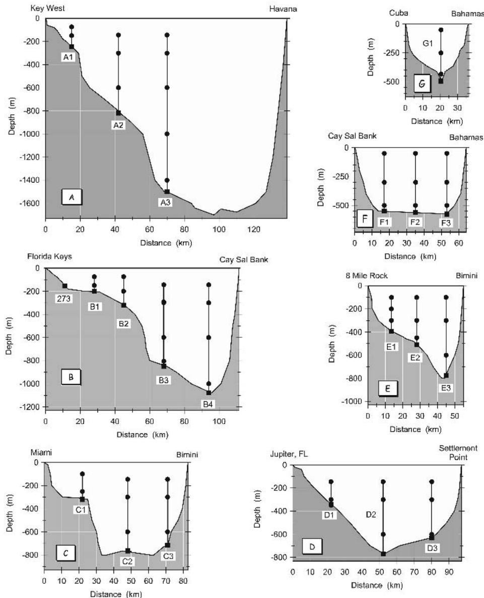
FIG. 2. Channel cross sections (see Fig. 1) showing the moorings and distribution of instruments.
