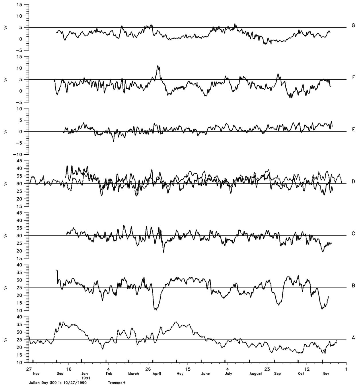
FIG. 5. Transports calculated from current-meter records (solid) and derived from cable measurements (dashed) for the indicated sections in the Straits of Florida.
