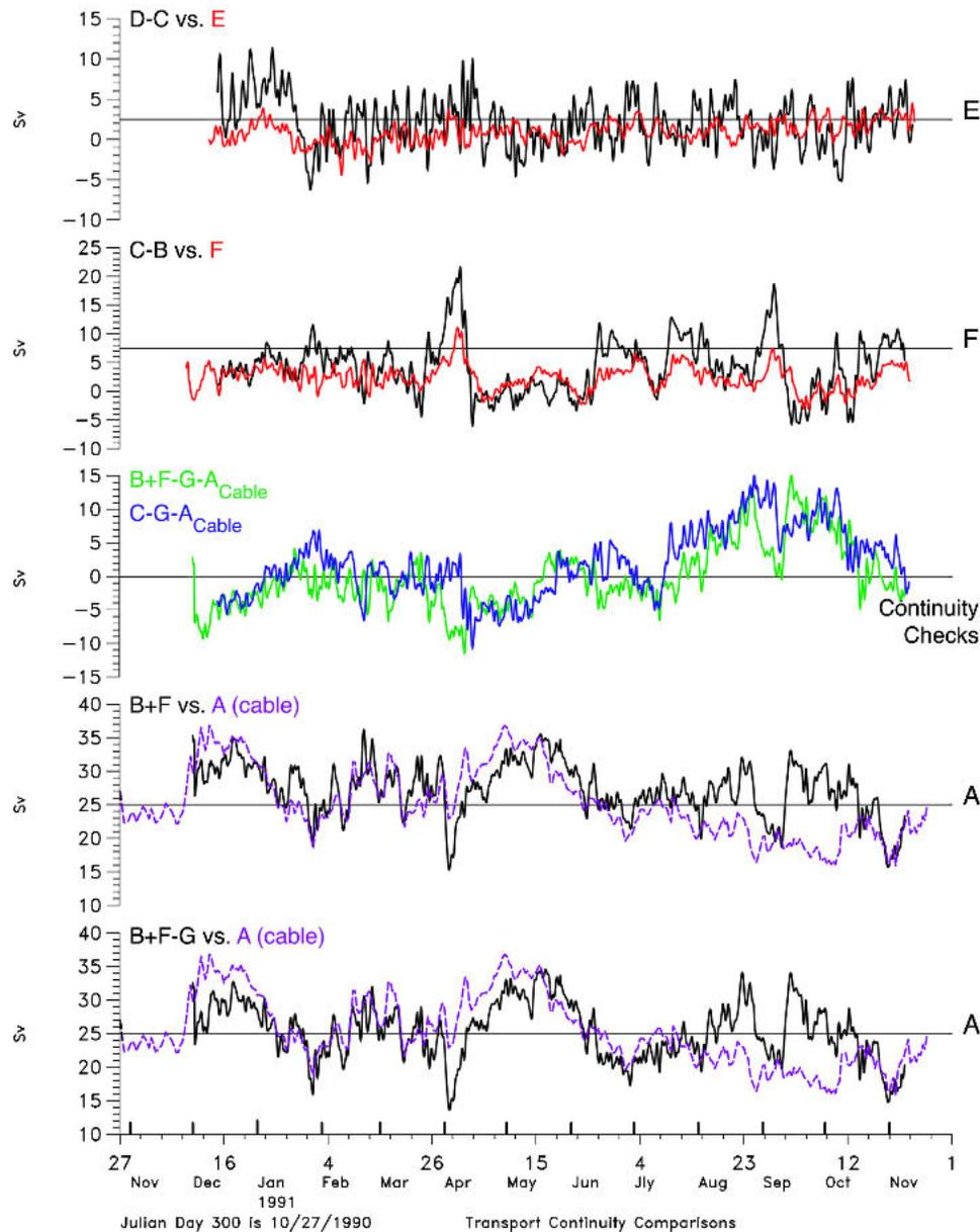
FIG. 7. Comparisons of transports for the indicated sections estimated by sum and difference (solid black), cable (dashed purple), and directly from current meters in the section (solid red). Here  $B + F - G$  is the estimate of transport across A using continuity. Continuity mismatches between the transports for the cable (A) and sections B + F (green) and C (blue) are given in the center panel.
