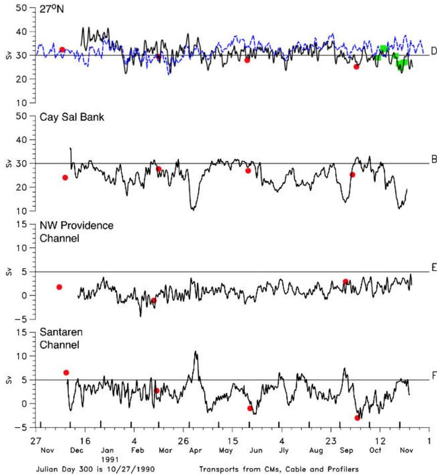
FIG. 4. Transports from current velocities (black) for the indicated sections. Red dots are transport estimates from Pegasus profiler sections. For section D, the red dots are the sums of the profiler measurements for channels B + F + E. Green squares are transports from NOAA–AOML dropsonde sections at 27°N, and the blue dashed line is the transport from the West Palm Beach to Eight Mile Rock cable.
