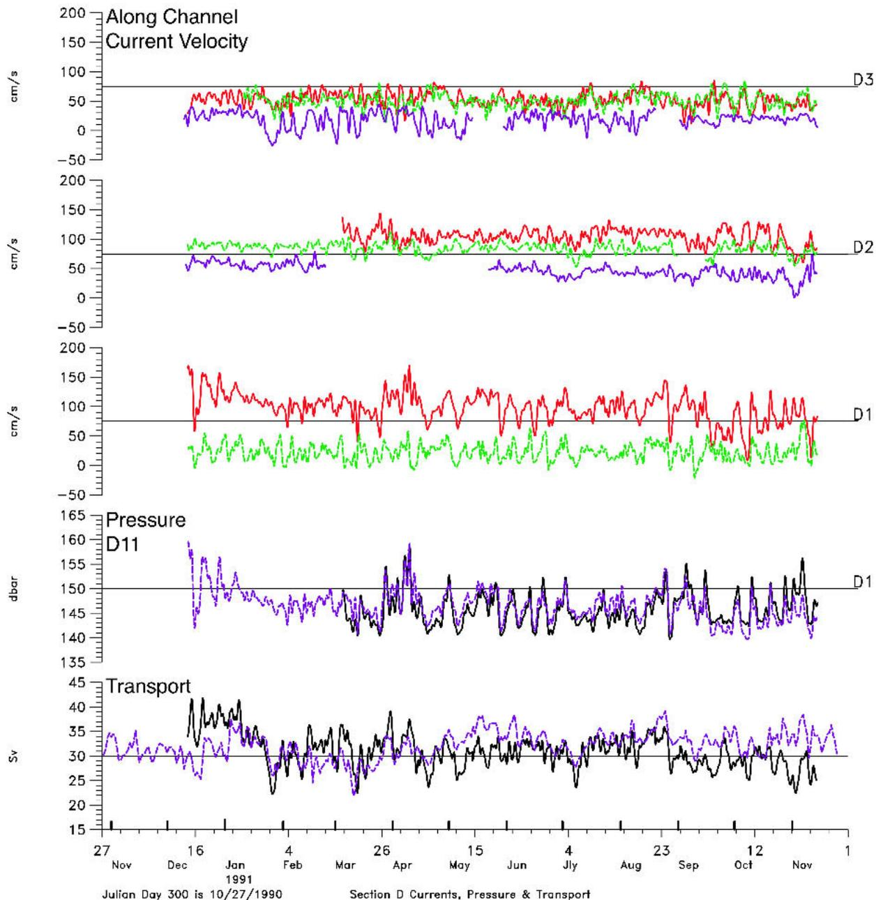
FIG. 3. Top three panels show along-channel 40-HLP velocities at the indicated moorings on section D. Nominal depths are 145 (red), 300 (green dashed), and 600 m (purple). Depth of the 145-m instrument on D1 as measured (solid black) and estimated (purple dashed), and the calculated (solid black) and cable-derived transports (purple dashed) are on the bottom two panels, respectively.
