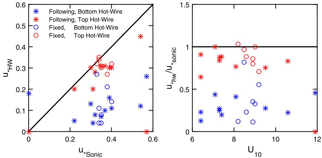
FIG. 1. (left) The  $u_*$  measured by hot wires near the surface vs  $u_*$  measured by the sonic anemometer at 4.6-m height. (right) Ratio of the hot-wire and sonic-anemometer  $u_*$  vs  $U_{10}$ . In both panels, asterisks indicate the following mode and circles the fixed mode, and blue indicates the bottom hot wire and red the top hot wire. Note that the top hot wire is always stationary.
