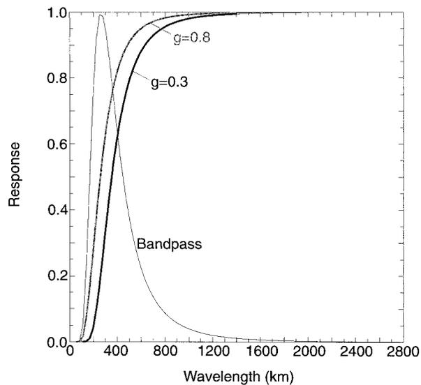
FIG. 1. Response curves vs wavelength (km) for objective analyses used in the cold pool identification procedure. Curves  $g = 0.3$  (thick black line) and  $g = 0.8$  (thick gray line) are the large and mesoscale analyses, respectively, used to define the mesoscale bandpass filter (thin solid line).
