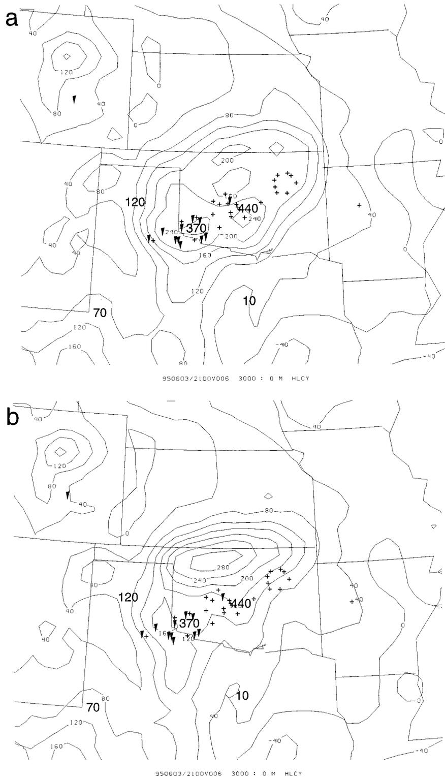
FIG. 11. SREH ( $\text{m}^2 \text{s}^{-2}$ ) from (a) cold pool run and (b) control run at 6 h into the model forecasts valid 2100 UTC 3 Jun 1995. Contour interval is  $40 \text{ m}^2 \text{s}^{-2}$ . Numbers in bold indicate SREH values calculated from the VORTEX special soundings. An inverted triangle indicates a tornado report, while a + indicates the location of a severe wind report.
