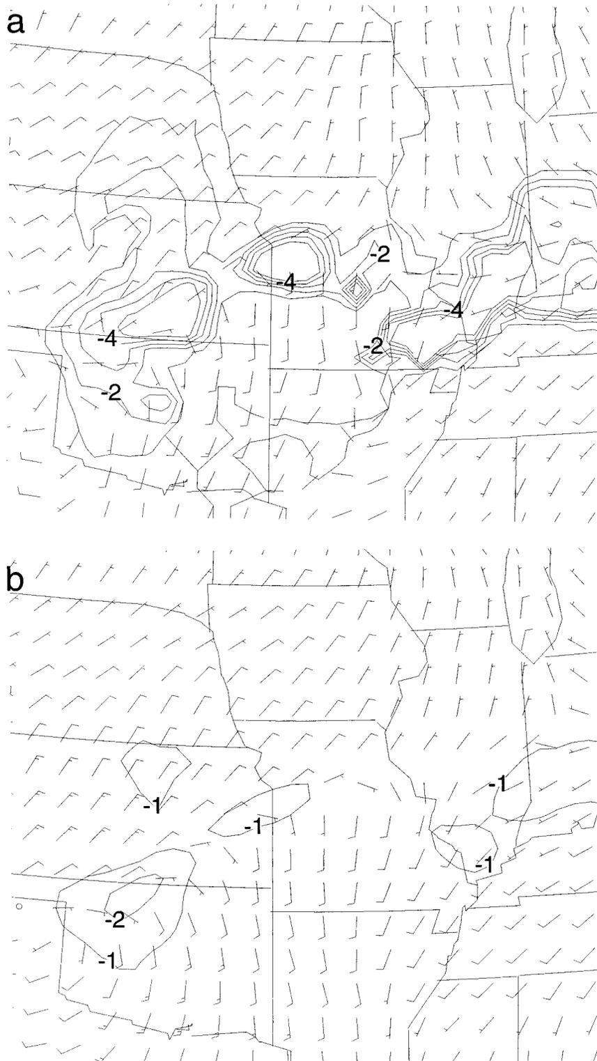
FIG. 9. Differences in 2-m temperatures ( $^{\circ}\text{C}$ ) from the cold pool and control runs valid at (a) 3, (b) 6, and (c) 9 h into the model runs started at 1200 UTC 17 May 1995. Negative values indicate that the cold pool run is colder than the control run. Contour interval of  $1^{\circ}\text{C}$  in (a) and
